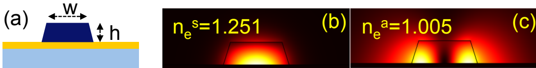
Figure 4.3: (a) Opto-geometrical parameters for the finite-element analysis of an un-doped DMI waveguides, W = 900\text{nm} , h = 400\text{nm} (see Fig. 4.3(a)), n_{\text{PMMA}} = 1.489 , n_{\text{Au}} = 0.57 + i11.7 for a wavelength of \lambda_o = 1580\text{nm} . The trapezoidal shaped cross-cut of the DLSPW accounts for the undercut of the vertical side-walls produced by PMMA processing. (b) (resp. (c)) Spatial distribution of the guided power for the fundamental symmetric (resp. higher-order anti-symmetric) DLSPW mode.
