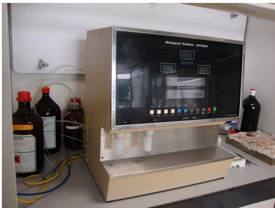
Photo II-3. Biological oxidizer-500 for the measurement of non-extractable radioactivity
