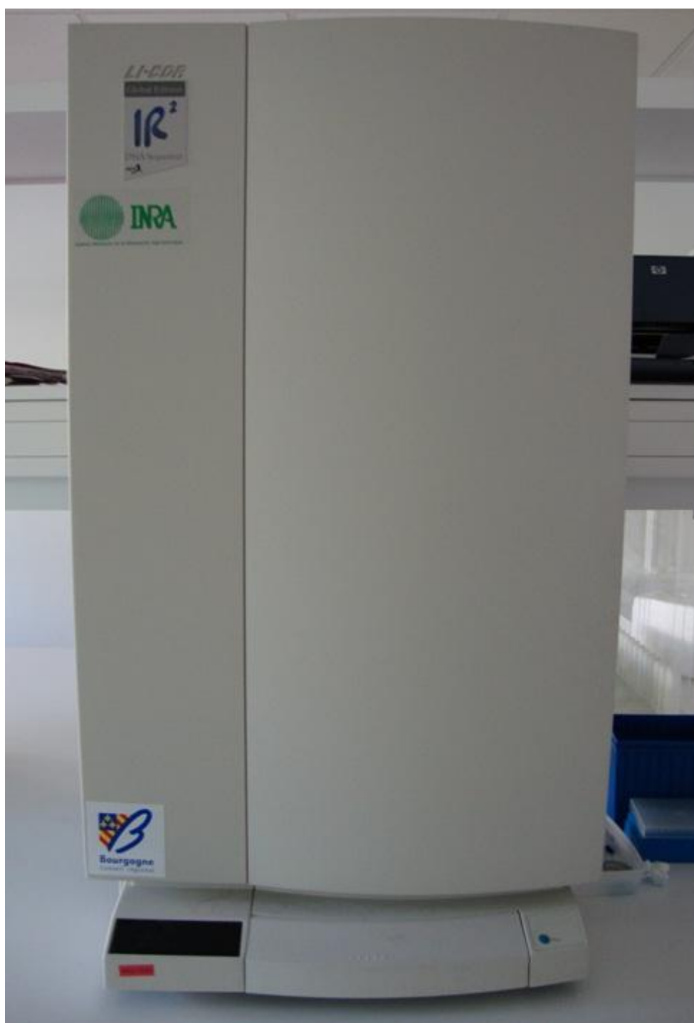
Photo II-7. LiCor (IR2, Bioscience) DNA sequencer for A-RISA fingerprinting
