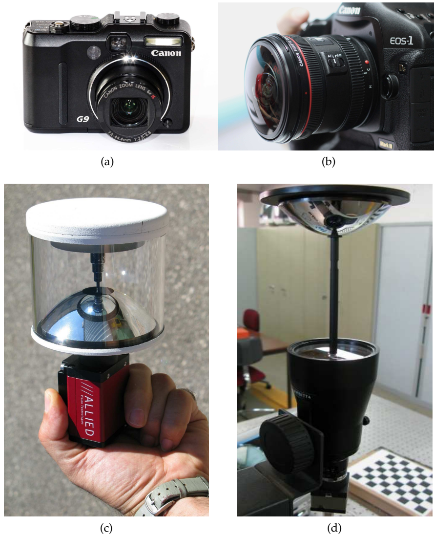
Figure 12: Four different categories of sensors used in this thesis. (a) Perspective camera. (b) Camera with fisheye lens. (c) Camera with folded optics. (d) Paracatadioptric system composed of a parabolic mirror in front of a telecentric lens.
