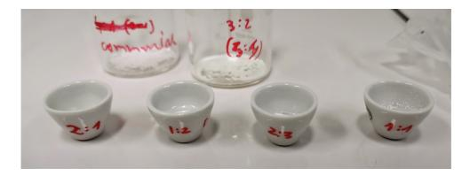
Figure 3.15: Containers used for the synthesis of BiCit by aging. The process was performed in small crucibles, beakers, and Petri dishes, placed for the time of synthesis in a desiccator.
