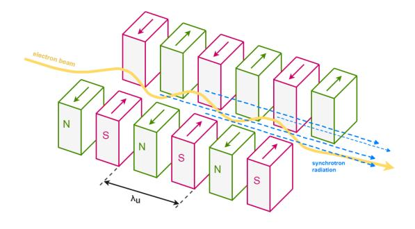
Figure 2.7: A schematic representation of an insertion device. Depending on the value of magnetic field and distances in between magnets ( $\lambda_u$ ), as well as the amount of magnets used. The magnets face the opposite poles, and are placed alternately in their rows. A scheme can represent either a wiggler or an undulator.
