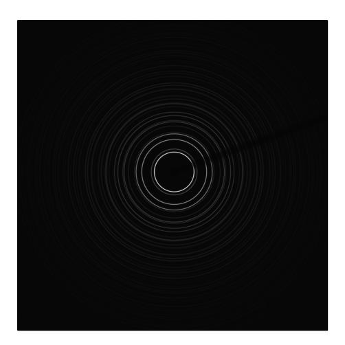
Figure 5.4: A detector image of CeO<sub>2</sub> calibrant rod. The image was measured in PETRA-III, at a Swedish Materials Science Beamline (P21.1). The diffraction cones and shadow of a beamstop are clearly visible. The calibration process transforms the 2D image into a 2D plot.
