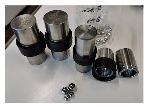
Figure 2.2: A photograph of the milling jars and the stainless steel balls used in the project. During the synthesis, the reaction mixture is placed inside one half of the jar, and followed by the milling balls. Then, the jar is sealed with the other half and the rubber seal. The assembled jars are placed vertically in between the clamps of the mill, before the milling starts.
