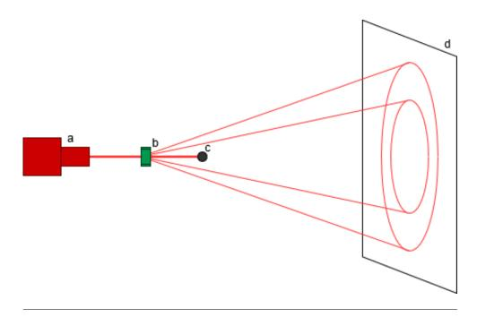
Figure 2.5: A schematic representation of diffraction cones generation. An initial Xray beam is produced by the source (a) and directed through a polycrystalline sample (b), to then be caught by a beamstop (c). Some of the initial beam is diffracted in a form of the Debye-Scherrer diffraction cones. When gathered by a 2D detector, they form the diffraction rings that are associated with specific a family of diffracting planes.
