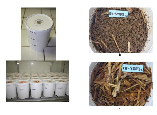
**Fig. 1**: Microcosms were incubating at 15°C in a climatic chamber (a). Straw was mixed with the soil in one half microcosms (b) while it was left at the surface of soil in the other half (c).
