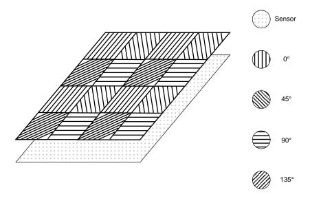
FIGURE 2.1: Illustration of a DoFP polarization sensor micro-grid.
