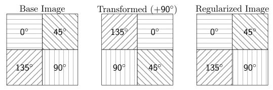
Figure 4.7: Illustration of the pixel grid of a rotated DoFP polarimetric camera.
