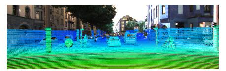
FIGURE 3.4: Illustration of LiDar point-cloud<sup>2</sup>. Sparsity can be observed as well as erroneous estimation on vehicle windows.
