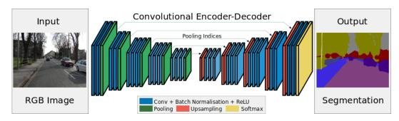
FIGURE 4.13: Illustration of SegNet architecture.
