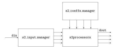
FIGURE 4.13: Dataflow in s2c2. The data arriving to the module is handled by s2\_input\_manager, which make it manageable for the s2processors. The latter also gets the pre-learnt filter needed for the pattern-matching operations from s2\_coeffs\_manager in parallel, and perform the computations. Once it is over, the data is sent in parallel to the dout output port, which feed the next processing module.
