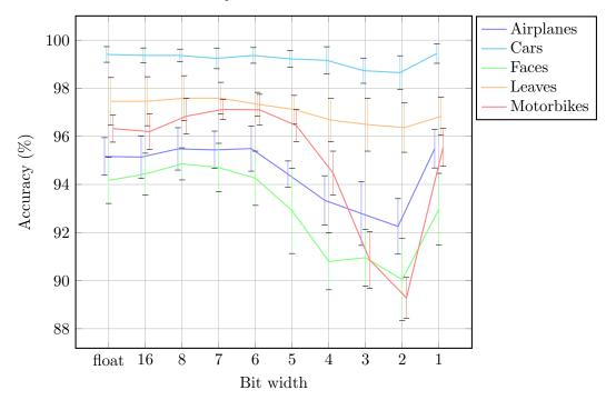
HMAX accuracy w.r.t Gabor filter bit width
