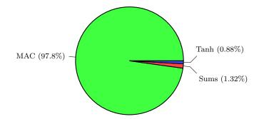
FIGURE 3.5: Complexity repartition of the CFF algorithms, separated in three types of computations: MAC, hyperbolic tangents ("Tanh") and sums. We see here that the large majority of operations are MAC, toward which most effort should then be put for fine optimizations or hardware implementation.
