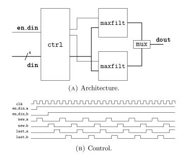
FIGURE 4.11: clunit. Figure 4.11a shows the principle components of the module architecture, and Figure 4.11b shows the control signals enabling and disabling the data.
