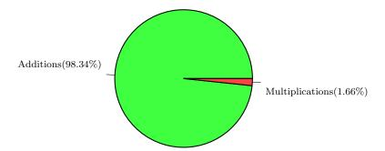
FIGURE 3.3: Complexity repartition of Viola and Jones' algorithm when processing a 640 × 480 with a 24 × 24 sliding window. From Equations 3.7 to 3.13, we see that the integral image computation requires 2WH additions, the feature extraction needs  $\overline{N_{\text{op}}}N_fN_w$  additions, and  $C_{\text{VJ}_N}$  needs WH multiplications and 2WH. Thus, we need a total of  $4WH + \overline{N_{\text{op}}}N_fN_w$ .
