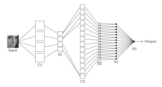
FIGURE 3.4: Convolutional Face Finder [50]. This classifier is a particular topology of a ConNet, consisting in a first convolution layer C1 having four trained convolution kernels, a first sub-sampling layer S1, a second convolution layer C2 partially connected to the previous layer's units, a second sub-sampling layer S2, a partially-connected layer N1 and a fully-connected layer N2 with one output unit.
