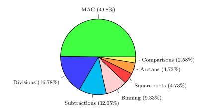
FIGURE 3.16: Complexity repartition of HOG features extraction.
