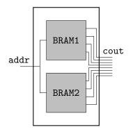
FIGURE 4.7: coeffs\_manager module. In order to simplify the process, all coefficients needed at a particular time are read all at once from several BRAM, of which only two are represented here for readability. The coefficients are then concatenated in a single vector directly connected to the cout output port.
