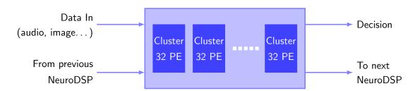
FIGURE 1.3: NeuroDSP architecture [5]. A NeuroDSP device is composed of 32 clusters, called *P-Neuro*, each constituted of 32 artificial neurons called PE, thus representing a total of 1024 neurons. The PEs may be multiplexed, so that they can perform several instruction sequentially and thus emulate bigger neural networks. When timing is critical, one may instead cascade several NeuroDSP processors and use them as if it was a single device.
