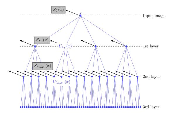
FIGURE 2.7: Invariant scattering convolution network [38]. Each layer applies a wavelet decomposition  $U_{\lambda}$  to its inputs, and feed the next layer with the filtered images  $U_{\lambda}(x)$ . At each layer, a low-pass filter is applied to the filtered images and the results are sub-sampled. The resulting so-called "scattering coefficients"  $S_{\lambda}(x)$  are kept to form the feature vector.
