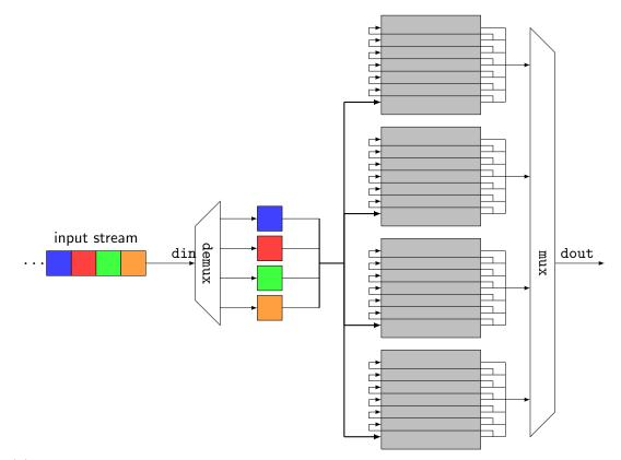
(B) s2\_handler module. Orientations are first demultiplexed, and written in parallel into the relevant s2\_pix\_to\_stripe, shown here in gray. There is one s2\_pix\_to\_stripe per scale in C1 feature maps -i.e 8. The output of those compinents are then routed to the dout output port, using a multiplexer.
