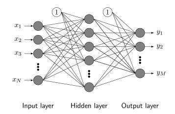
FIGURE 2.3: Multi-layer perceptron with one hidden layer.
