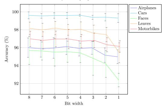
HMAX accuracy w.r.t input pixel bit width
