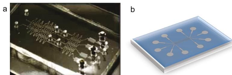
Figure 1.10 – (a) Microfluidics picture with complex channel design. Adapted from [47]. (b) Scheme of our microfluidic platform.
