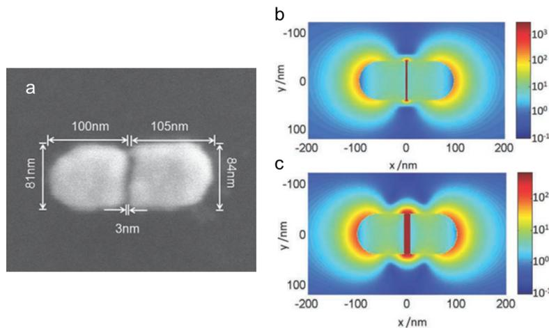
Figure 1.7 – (a) Lithographed Gold nanorods observed by SEM with a 42k x magnification. (b-c) FDTD calculation of the steady state field intensity distribution for dimer structure with 3 nm gaps (b) or 12 nm gaps (c). Adapted from [28].
