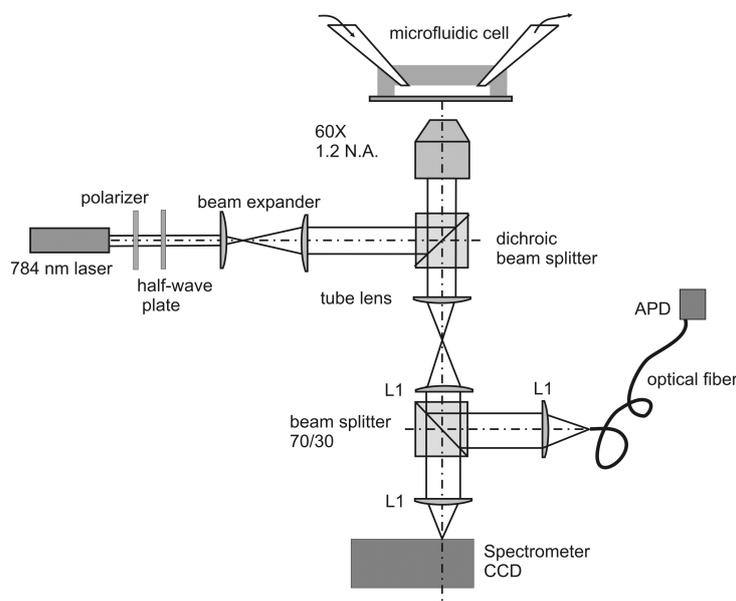
Figure 2.7 – Schematic representation of the confocal optical setup
