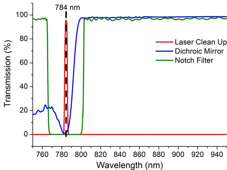
Figure 2.8 – Transmission characteristics of the different filters compound the filter cube.
