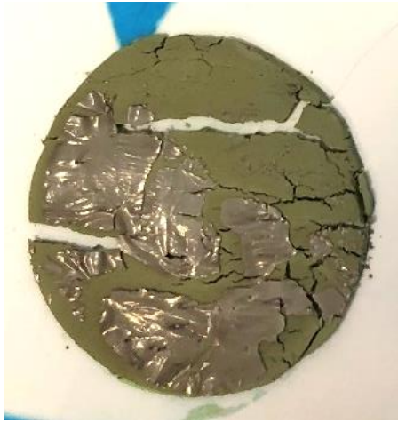
Figure E.1: Pictures of half-cell after co-sintering, the electrolyte layer is on the top side
