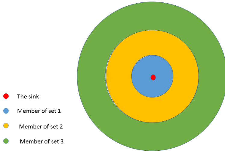
Figure 13: Top view of continuous set formation
