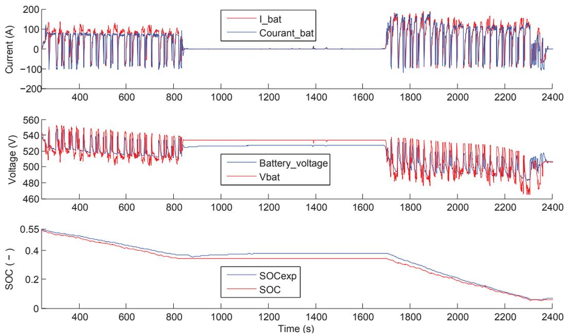
Figure 3.9: Verification of the battery model of the Noao car using quasi-static modeling method.
