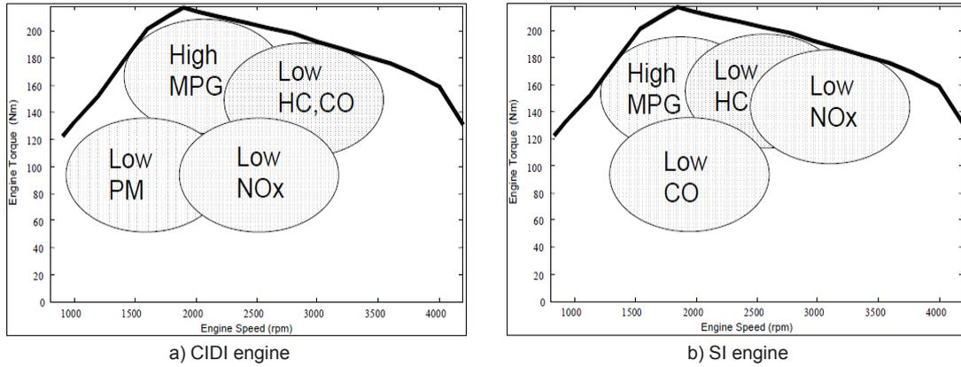
Figure 2.32: Fuel economy and emissions tradeoffs for; a) CIDI engine, and b) SI engine [45].
