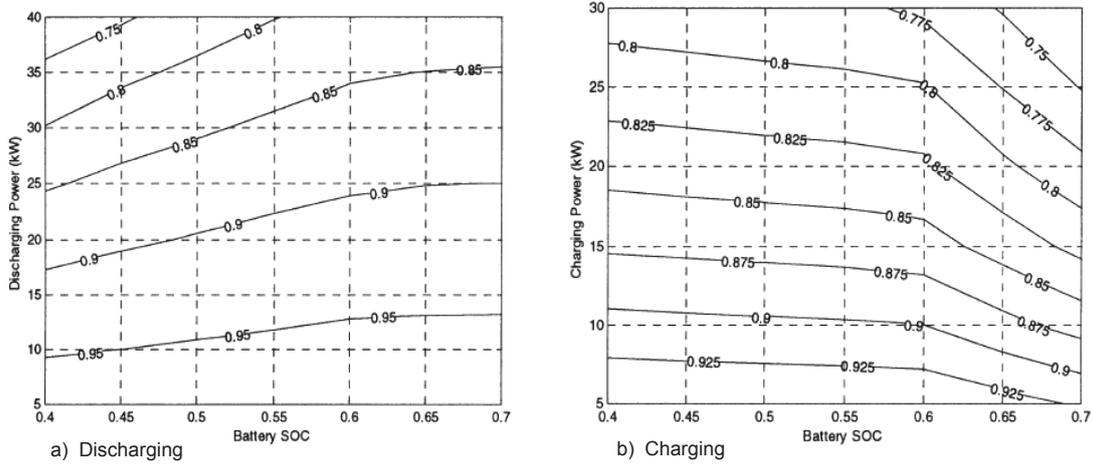
Figure 2.26: The efficiencies of the lead acid battery in function of power and SOC; a) Discharging, and b) Charging [42].
