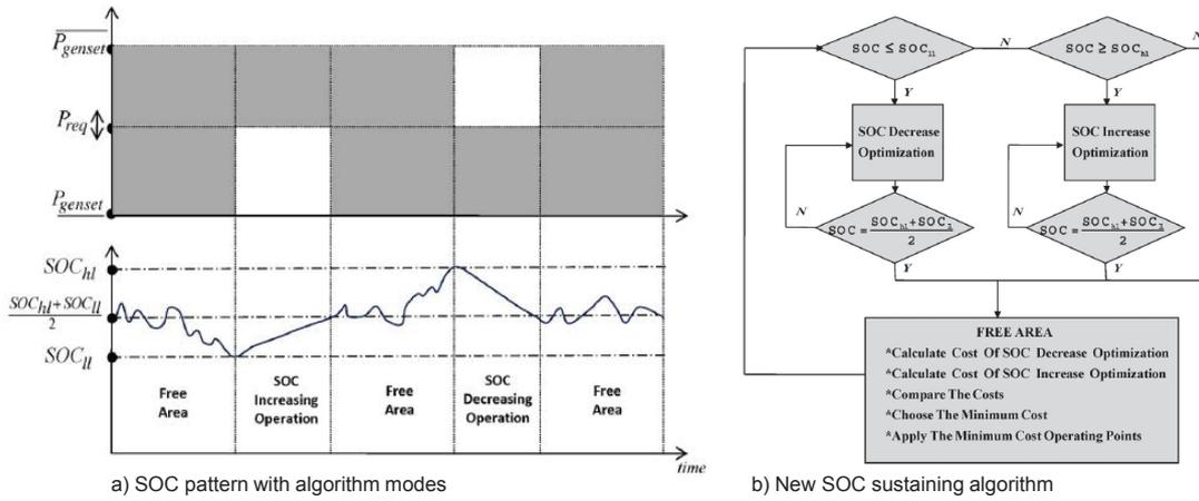
Figure 2.38: Schematic illustration of the new SOC sustaining ECMS algorithm; a) SOC pattern with algorithm modes, and b) New SOC sustaining algorithm [26].
