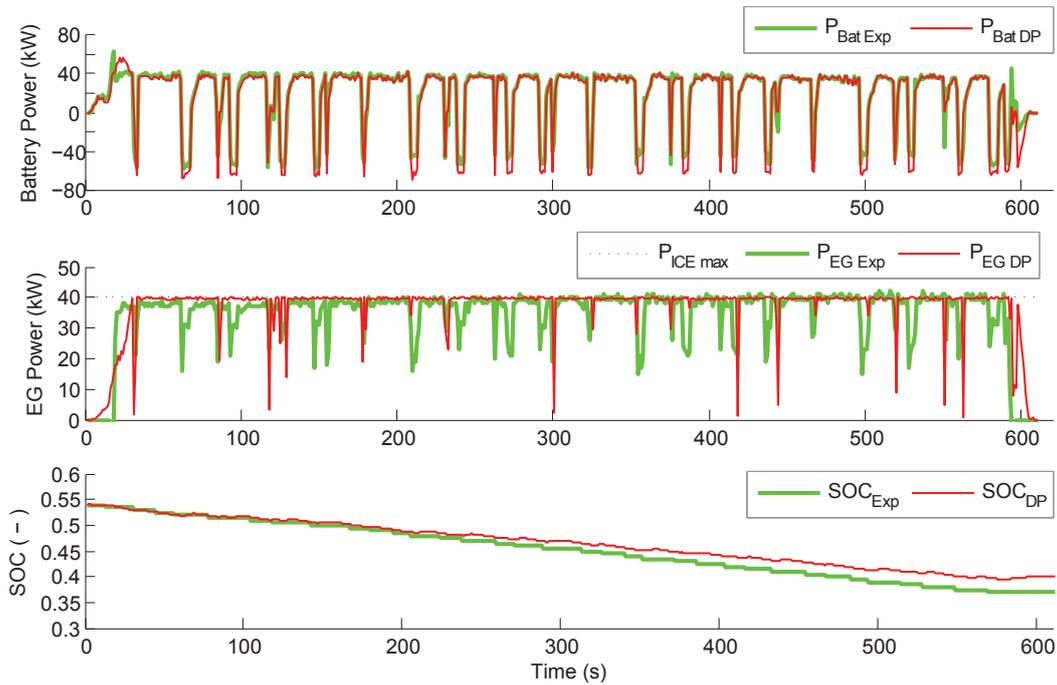
Figure 4.5: DP optimisation of the MC1 driving cycle for a longer autonomy.
