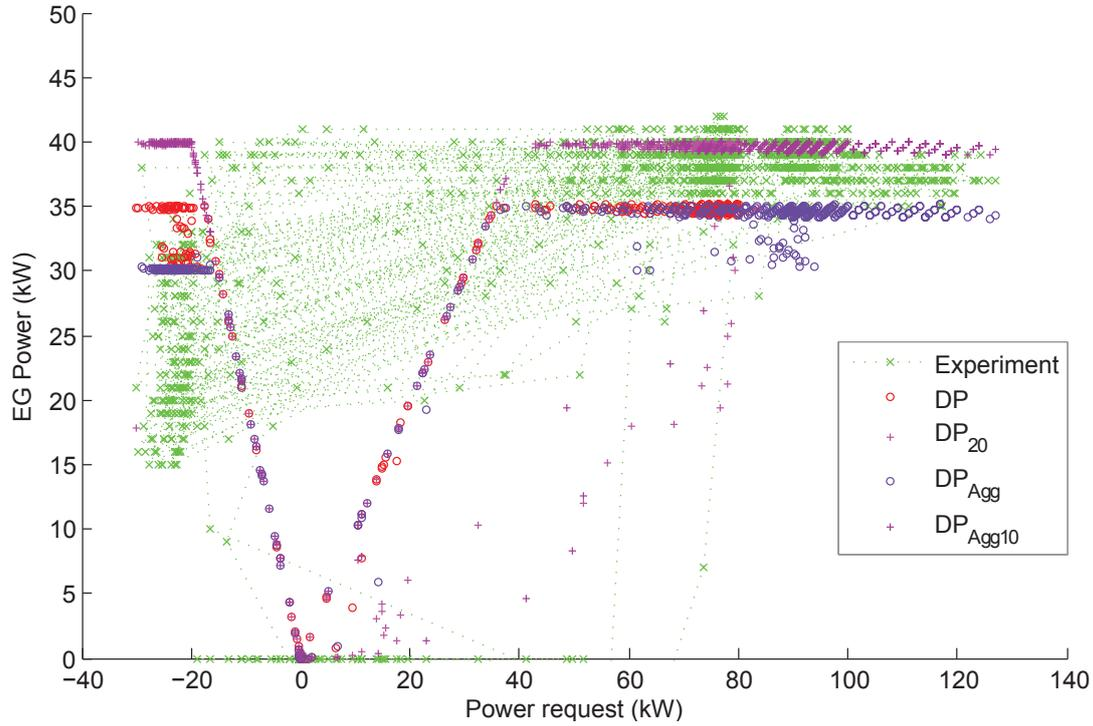
Figure 4.8: EG power in function of the power request.
