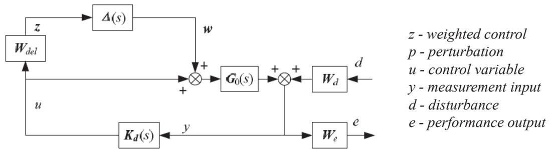
Figure 2.33: The EV driving control system with the uncertainty [33].
