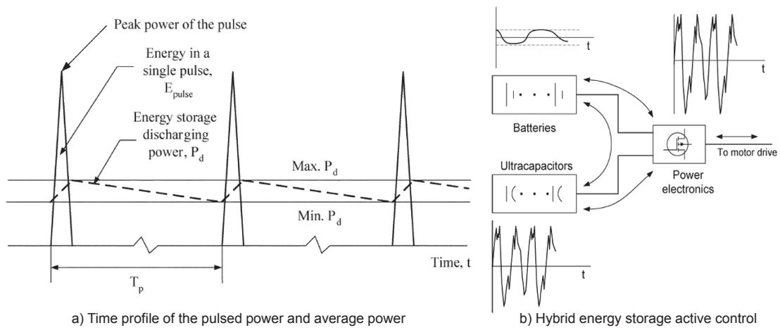
Figure 2.7: Conceptual illustration of; a) Time profile of the pulsed power and average power, and b) Hybrid energy storage active control [79].
