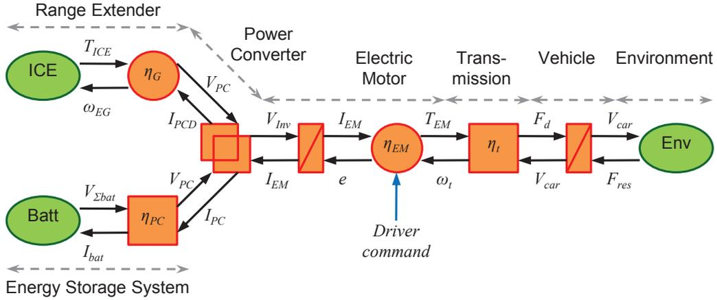
Figure 4.11: Energetic Macroscopic Representation of the car system to forecast driving cycles.
