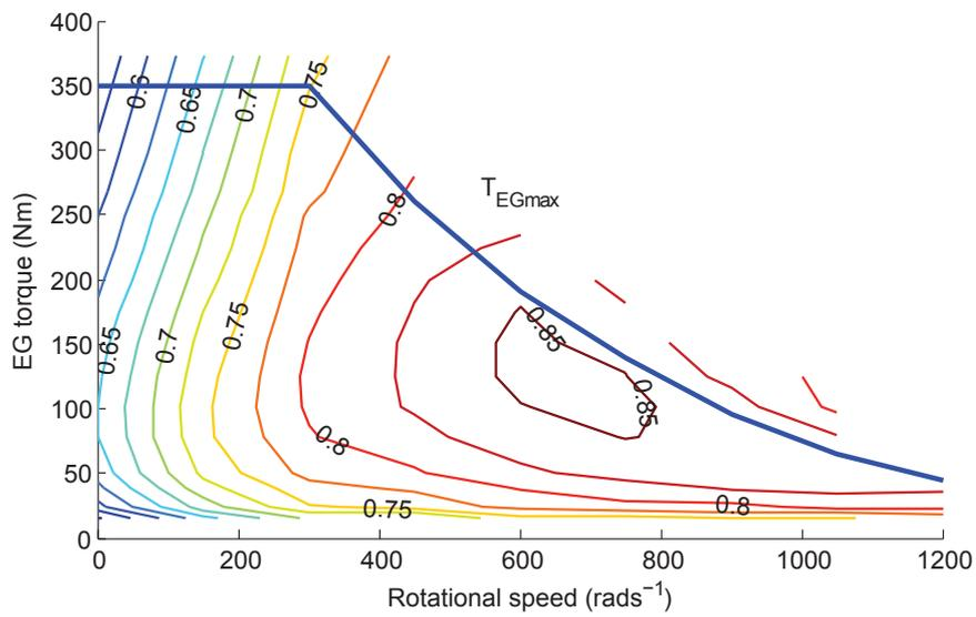
Figure 3.5: Electric generator efficiency map of the Noao car.
