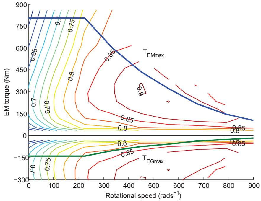
Figure 3.4: Electric motor efficiency map of the Noao car.
