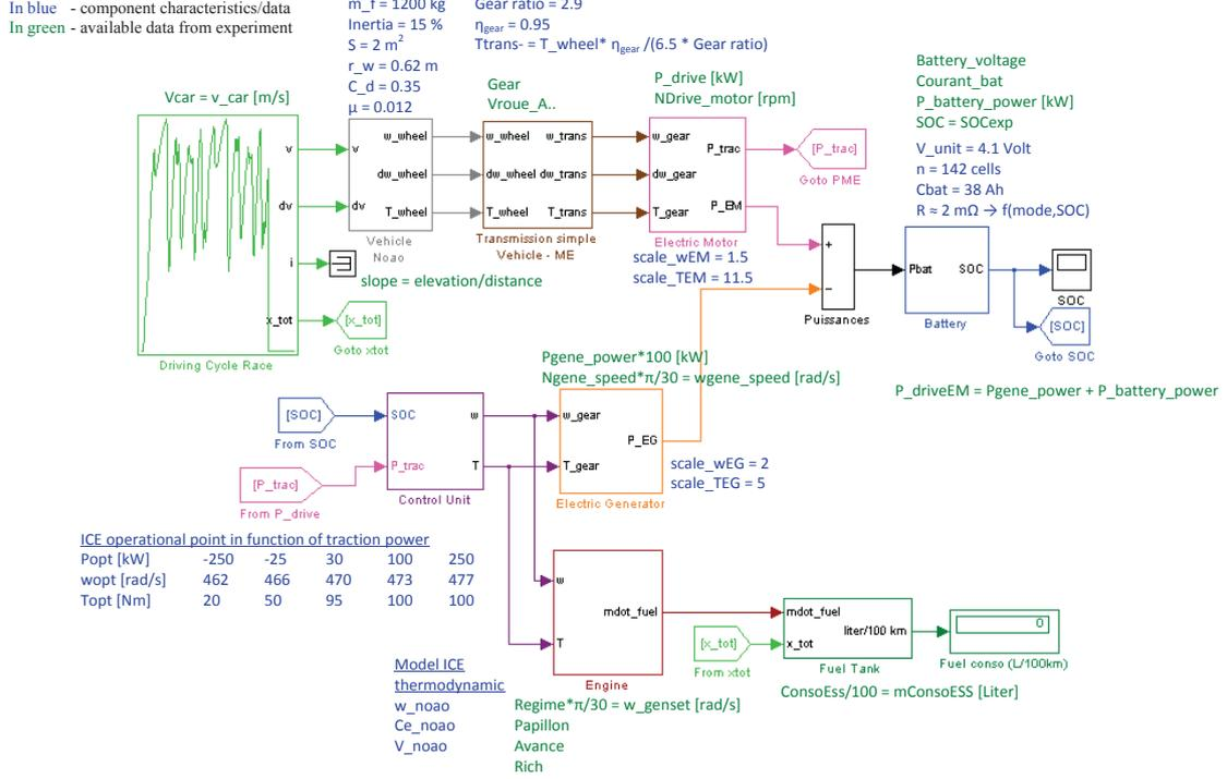
Figure 3.3: Modelisation of the Noao car using quasi-static modeling method.
