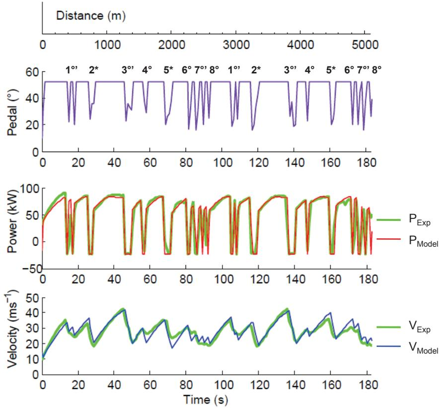
Figure 4.15: Comparison of the model with results from experiment for the small club circuit.
