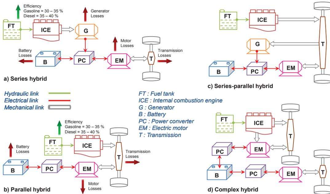
Figure 2.2: Diagrams of different HEV architectures, power flow, and power losses; a) Series, b) Parallel, c) Series-parallel, d) Complex
