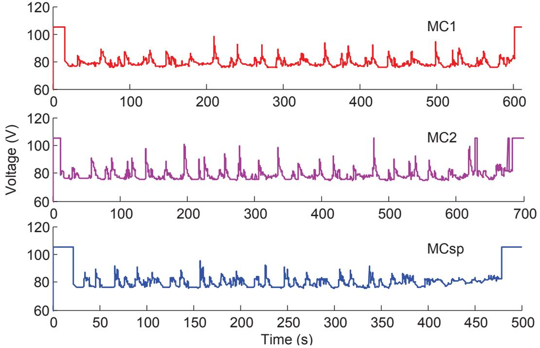
Figure 3.25: Voltage of the fuel cell stack in the racing car system for MC1, MC2, and MCsp driving cycles.
