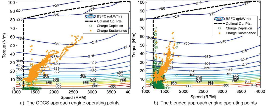
Figure 2.31: Comparison of; a) The CDCS approach engine operating points, and b) The blended approach engine operating points [76].
