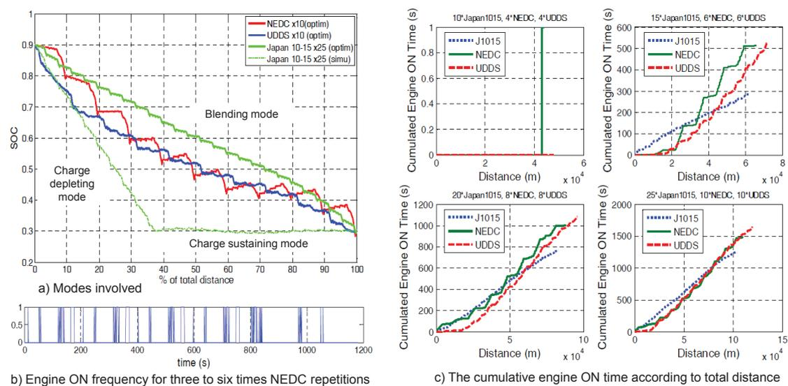
Figure 2.19: The control strategy; a) Modes involved, b) Engine ON frequency for three to six times NEDC repetitions, and c) The cumulative engine ON time according to total distance [91].
