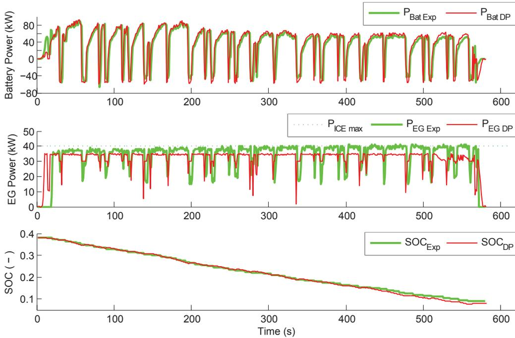
Figure 4.6: DP optimisation of the MC2, a more aggressive driving cycle of MC1.
