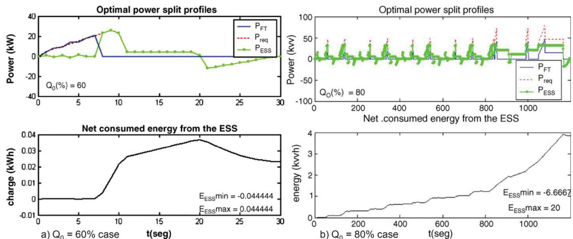
Figure 2.28: Results of power repartition of requested power ( $P_{req}$ ), between  $P_{ESS}$  and  $P_{FT}$  of  $Q_{nom} = 0.92$  Ah for; a)  $Q_0 = 60\%$  case, and b)  $Q_0 = 80\%$  case [95].
