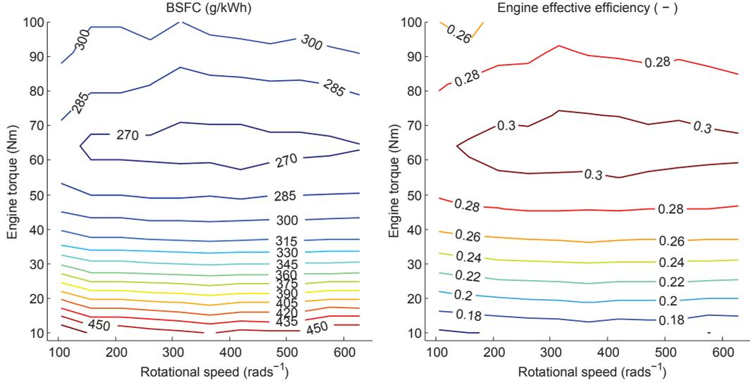
Figure 3.6: Internal combustion engine efficiency map of the Noao car.
