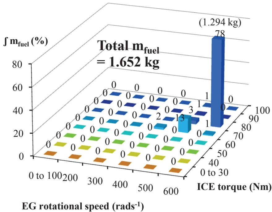
Figure 3.20: Percentage of the engine fuel consumption using the optimal control parameters.
