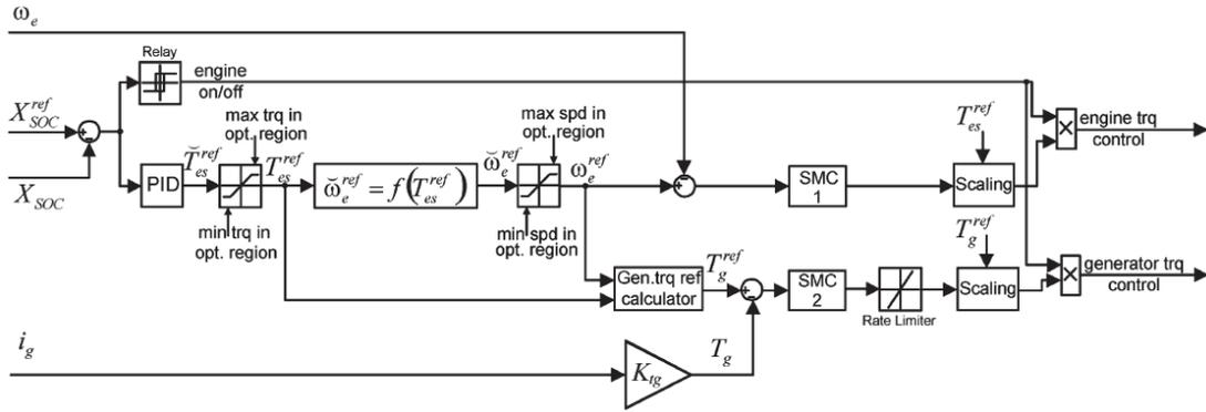
Figure 2.9: The block diagram of the auxiliary power unit (APU) controller based on two chattering-free SMC [80].
