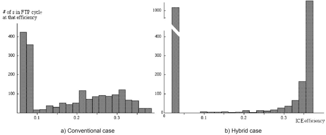
Figure 2.3: Comparison of the ICE efficiencies; a) Conventional case, and b) Hybrid case [40].
