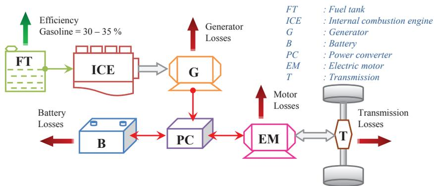
Figure 3.2: Architecture of the series hybrid.
