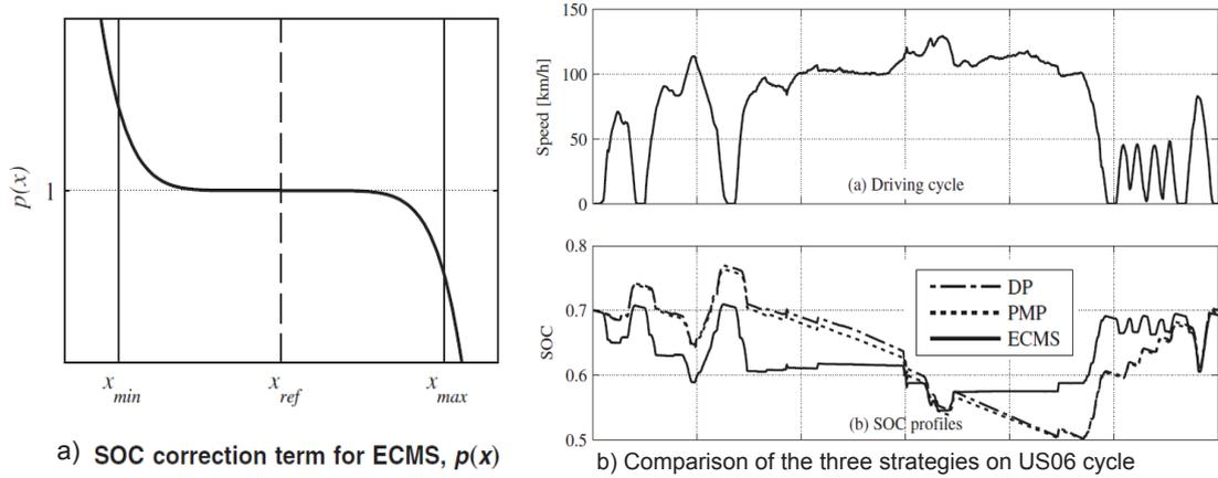
Figure 2.40: New ECMS control; a) SOC correction term for ECMS,  $p(x)$ , and b) Comparison of the three strategies on US06 cycle [7].
