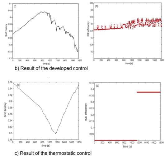
Figure 2.22: Comparison of the developed control strategy and the thermostatic control strategy; a) Concept of the thermostatic control, b) Result of the developed control, and c) Result of the thermostatic control [17].
