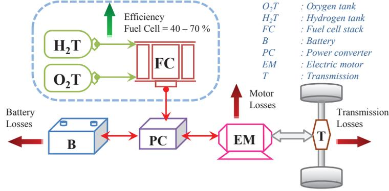
Figure 3.21: Architecture of the series hybrid vehicle system with fuel cell as range extender.
