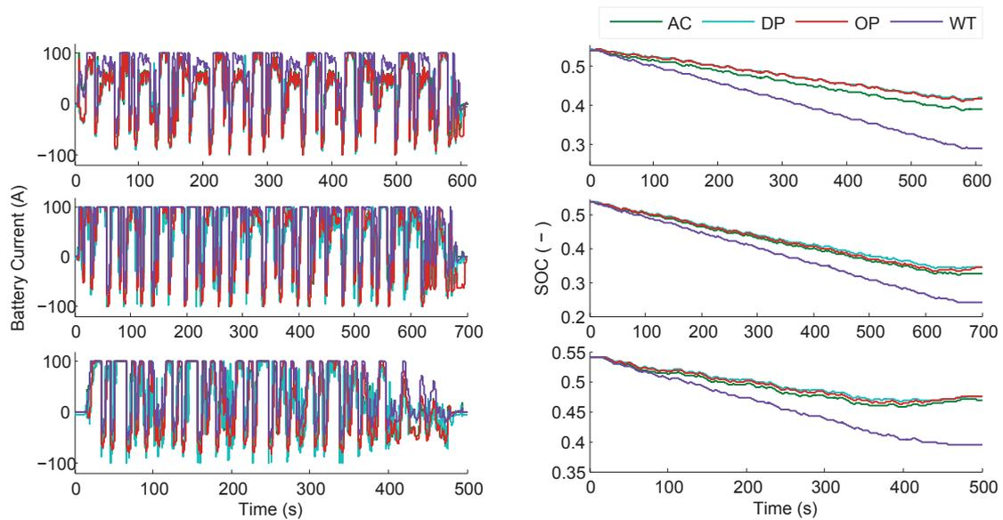
Figure 5.4: Results comparison of the battery current and SOC evolution of the race cycles (MCNoao1, MCNoao2, MCNoao3) for all four control strategies.
