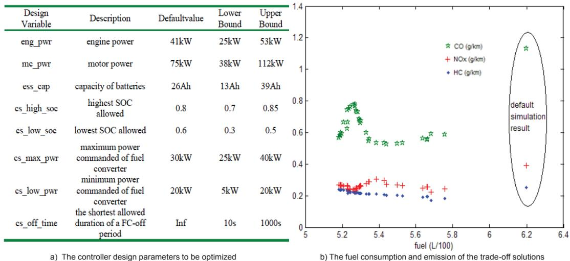
Figure 2.23: Multi-objective evolutionary algorithm; a) The controller design parameters to be optimised, and b) The fuel comparison of emission of the trade-off solutions [20].
