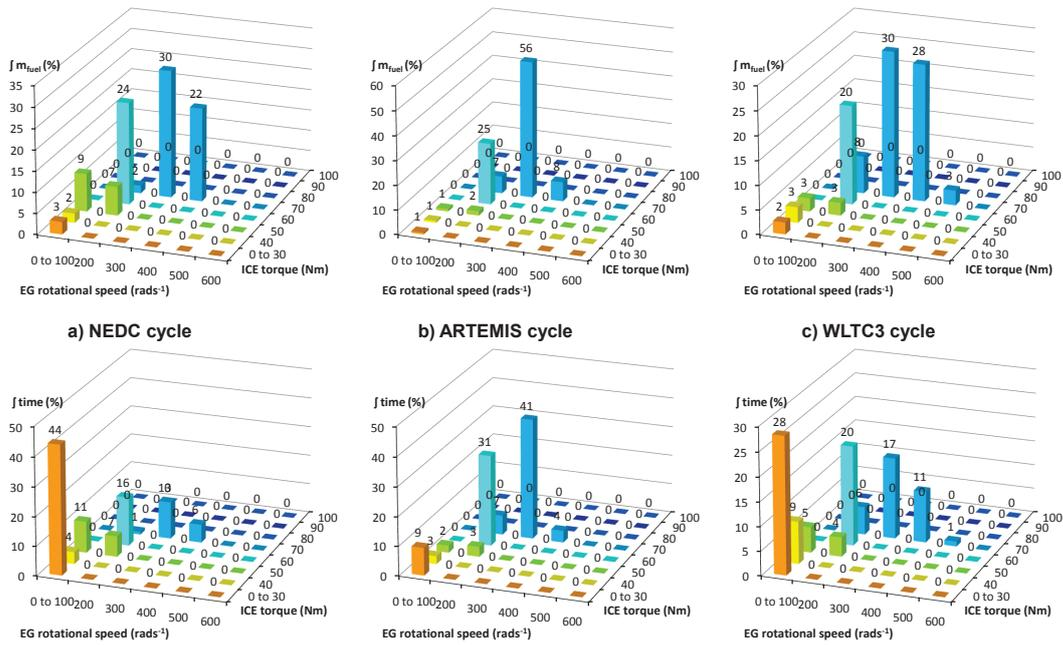
Figure 5.18: Percentage of ICE points distribution for the three road cycles; NEDC, ARTEMIS, and WLTC3 in terms of fuel consumption and time spent.
