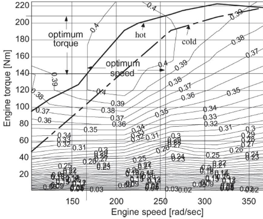
Figure 2.8: Engine efficiency map showing the optimal operating line [80].
