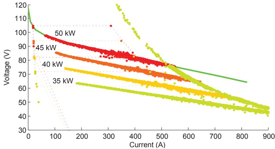
Figure 3.28: Operation points of the fuel cell stack using the same control strategy for the MC1 driving cycle.
