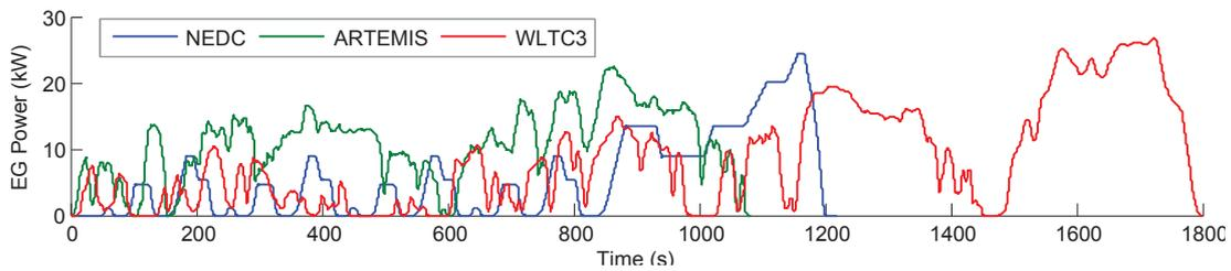
Figure 5.16: Given EG power for the three road cycles; NEDC, ARTEMIS, and WLTC3 under the modified optimal torque control strategy.
