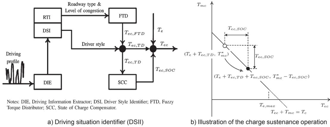
Figure 2.14: Architecture of IEMA; a) Driving situation identifier (DSII), and b) Illustration of the charge sustenance operation [77].
