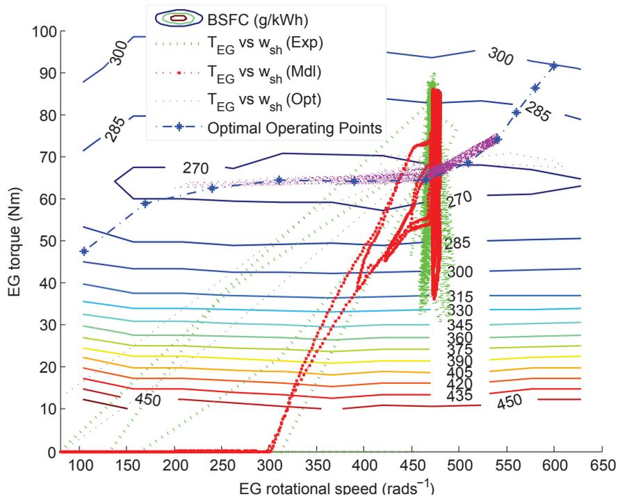
Figure 3.18: Engine operating points.
