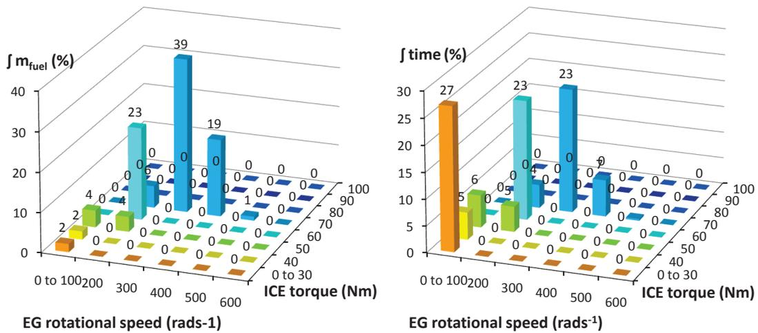
Figure 5.19: Percentage of average ICE points distribution for the three road cycles in terms of fuel consumption and time spent.
