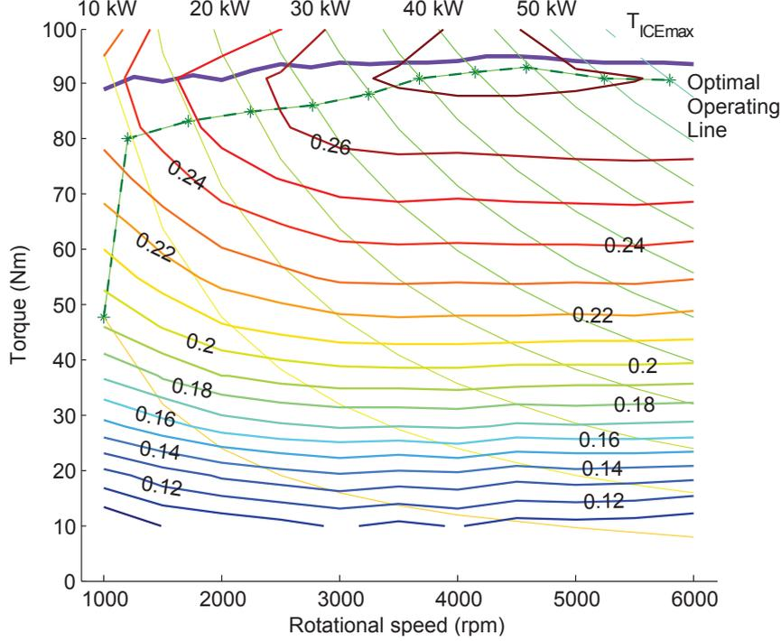
Figure 4.3: Optimal operating points on the combined engine and generator efficiency map.
