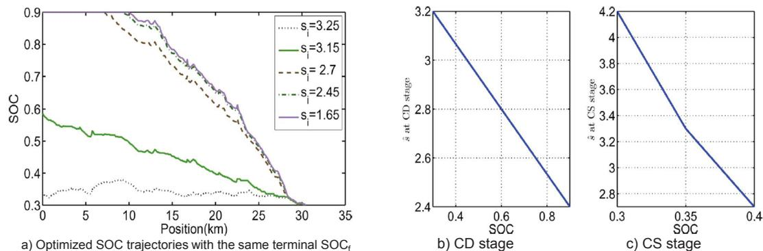
Figure 2.41: E-ECMS different initial guesses ( $s_i$ ); a) Optimized SOC trajectories with the same terminal  $SOC_f$ , and DS-ECMS estimated  $\hat{s}$  as a function of SOC at different stages; b) CD stage, and c) CS stage [28].
