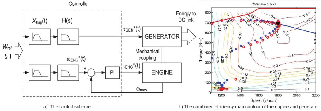
Figure 2.24: The trajectory optimisation control strategy; a) The control scheme, and b) The combined efficiency map contour of the engine and generator [25].
