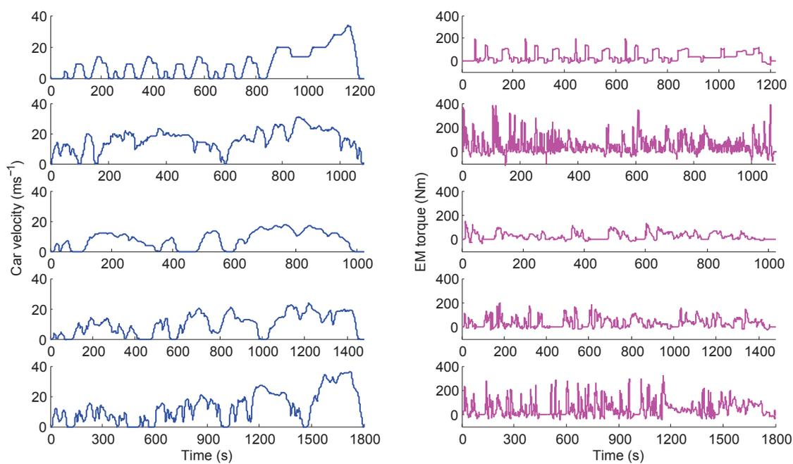
Figure 5.3: Road driving cycles (NEDC, ARTEMIS, WLTC1, WLTC2, WLTC3) and its EM torque request.
