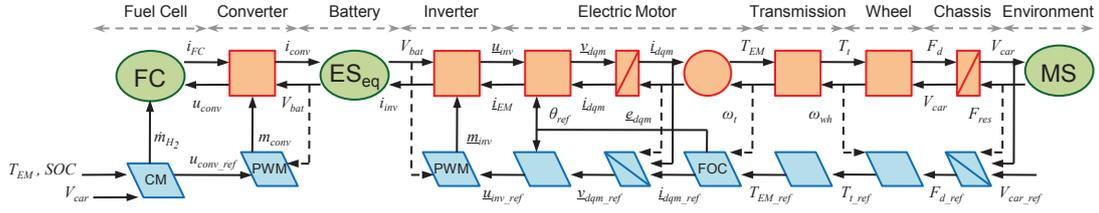
Figure 3.22: Energetic Macroscopic Representation and Inversion Based Control of the car system with fuel cell as the range extender.
