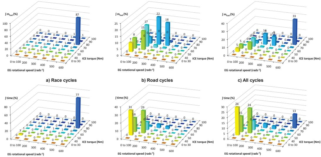
Figure 5.12: Percentage of ICE points distribution for the dynamic programming control in terms of fuel consumption and time spent.
