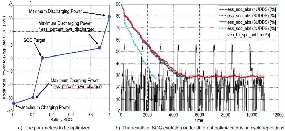
Figure 2.21: DIRECT algorithm; a) The parameters to be optimised, and b) The results of SOC evolution under different optimised driving cycle repetitions [30].
