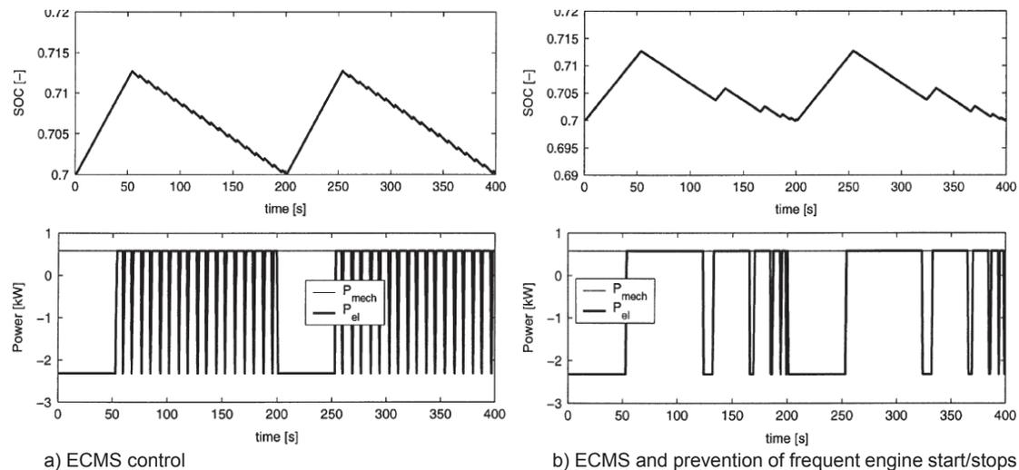
Figure 2.34: SOC evolution and number of startups before and after  $\Delta J_{ss}$  modification results; a) ECMS control, and b) ECMS and prevention of frequent engine start/stops [48].
