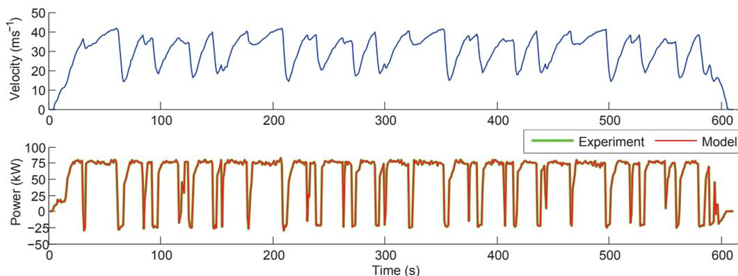
Figure 4.1: Magny Cours race driving cycle, MC1.
