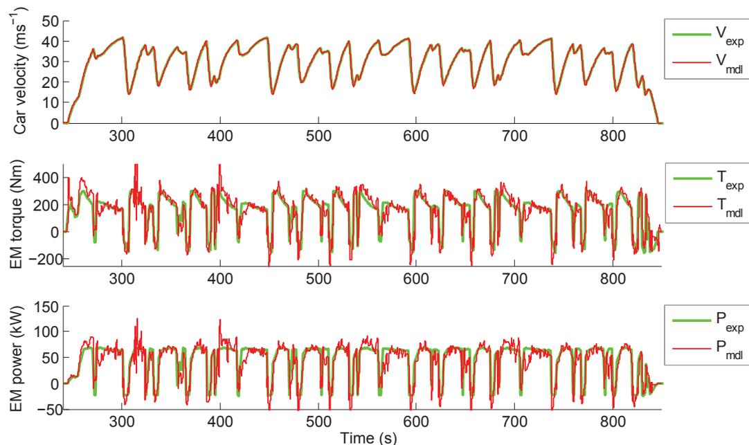
Figure 3.15: Driving cycle and profiles of power and torque at the electric motor.
