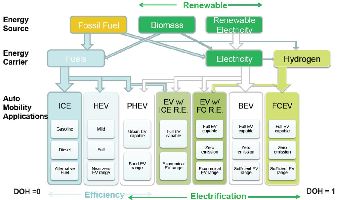
Figure 2.1: Schematic representation of HEV types with flow in power sources and design focus (extract from iTEC 2012 short course on HEV Fundamentals by M. Zhang) [27].
