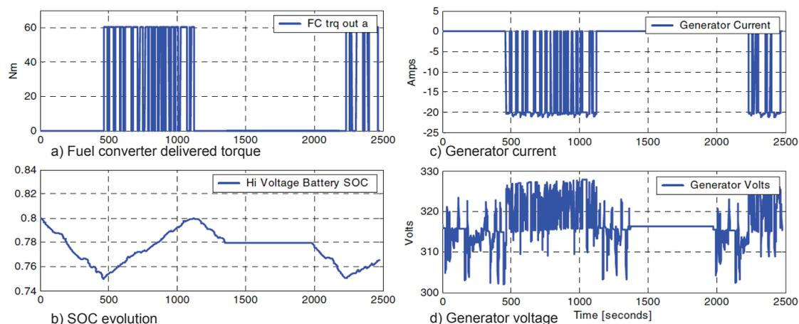
Figure 2.6: Result shows; a) Fuel converter delivered torque, b) SOC evolution, c) Generator current, and d) Generator voltage [55].
