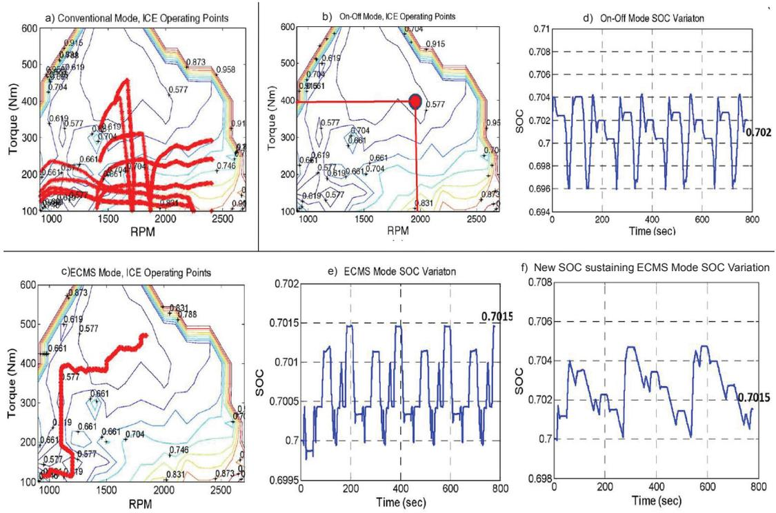
Figure 2.39: Comparison of ICE operating points on a combined map of  $k_1=0$ ,  $k_2=0.5$ ,  $k_3=0.5$ ,  $k_4=0$ , and  $k_5=0$  for; a) Conventional mode, b) On-Off mode, c) ECMS mode, and comparison of SOC variation between; d) On-Off control strategy, e) Classic ECMS mode, and f) New SOC sustaining ECMS mode [26].
