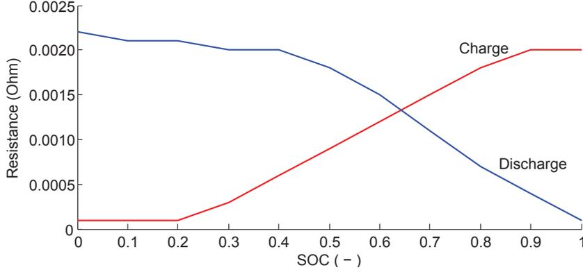
Figure 3.7: Resistance of the battery in function of SOC and its mode.
