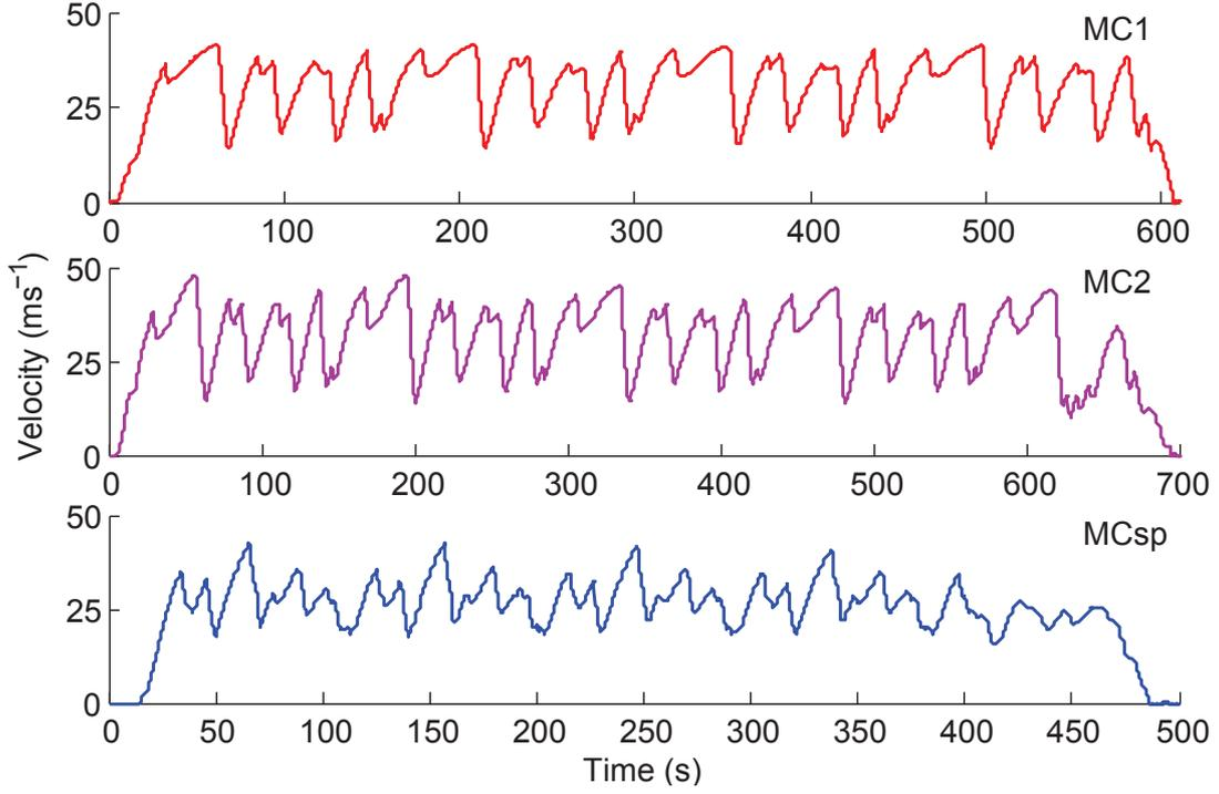
Figure 3.23: Driving cycles obtained from drive test of the racing car used for the case study; MC1, MC2, and MCsp.
