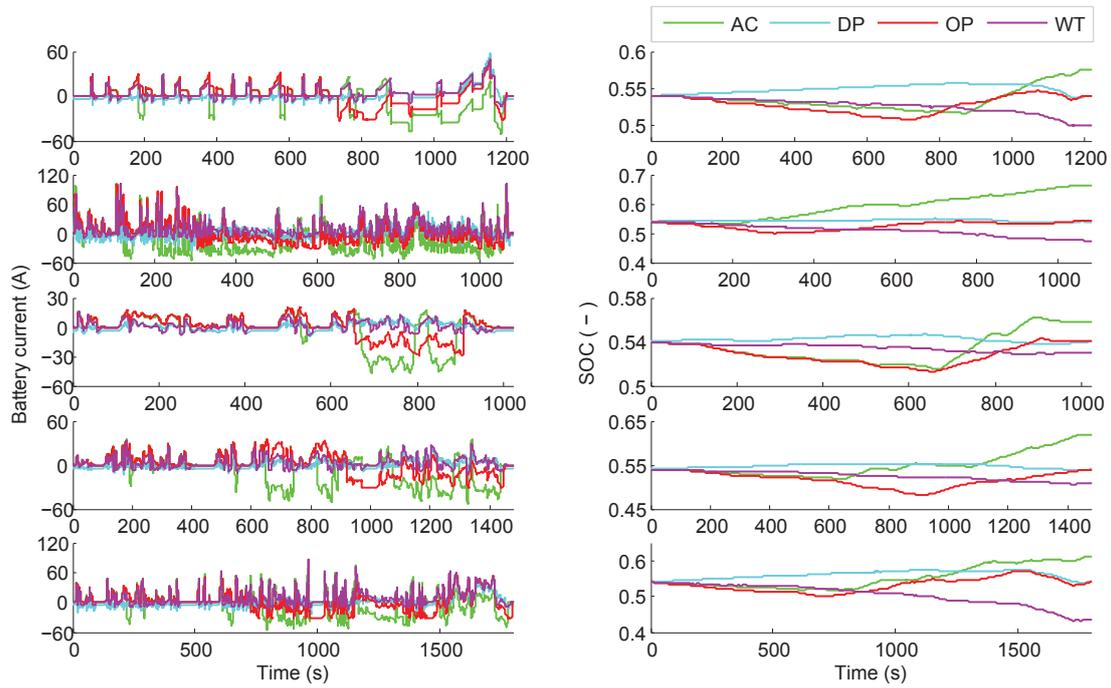
Figure 5.6: Results comparison of the battery current and SOC evolution of the road cycles (NEDC, ARTEMIS, WLTC1, WLTC2, WLTC3) for all four control strategies.
