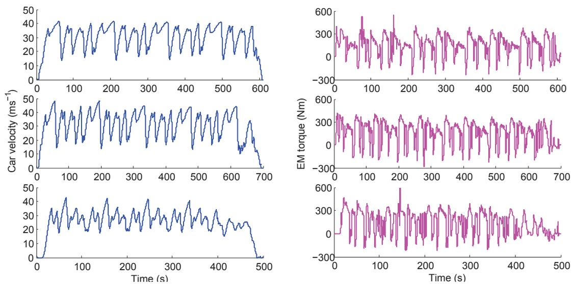
Figure 5.2: Race driving cycles (MCNoao1, MCNoao2, MCNoosp) and its EM torque request.
