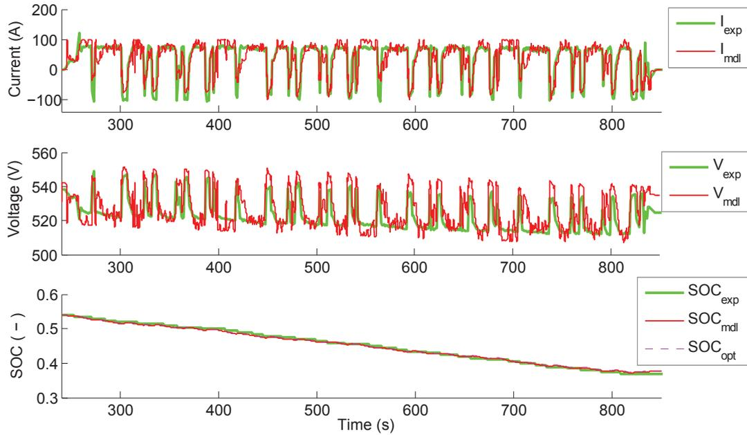
Figure 3.16: Results comparison of the current, voltage, and SOC evolution of the battery.
