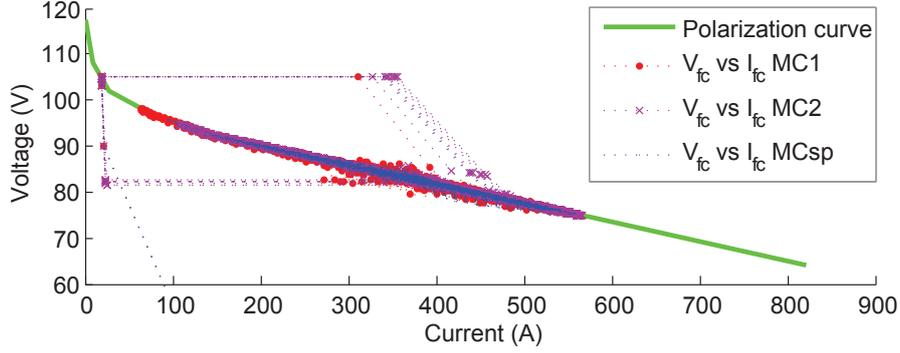
Figure 3.24: Polarization curve of the fuel cell stack and its operation points using the defined control strategy for the studied driving cycles.
