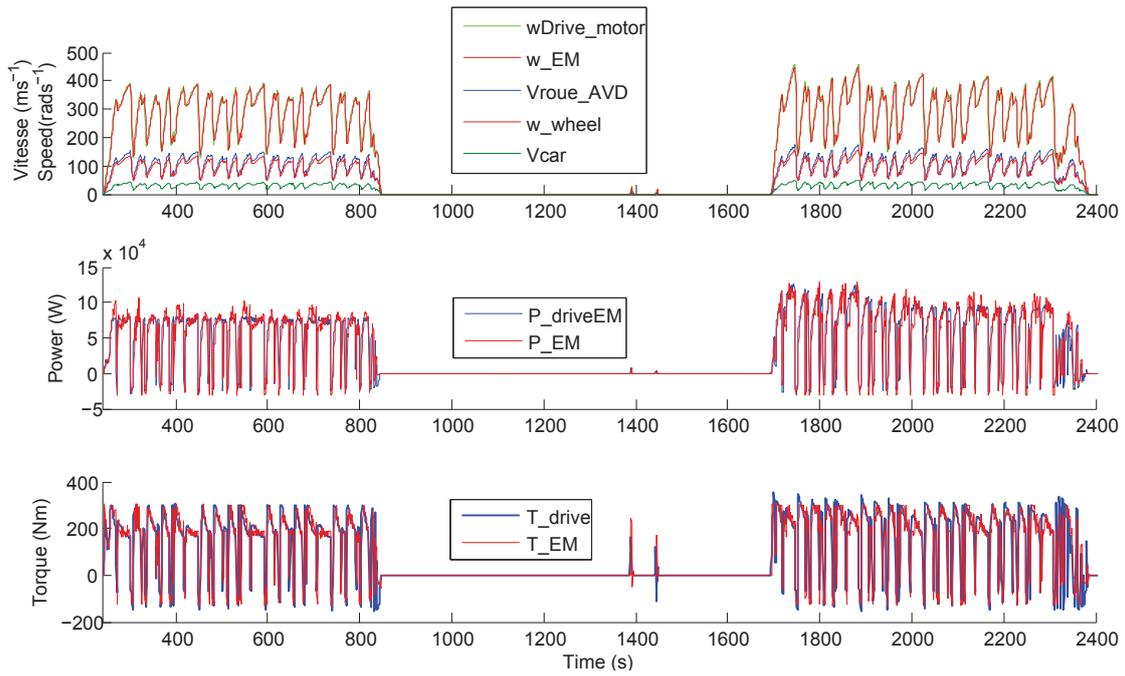
Figure 3.8: Verification of the traction model; chassis, wheel, and electric motor of the Noao car using quasi-static modeling method.
