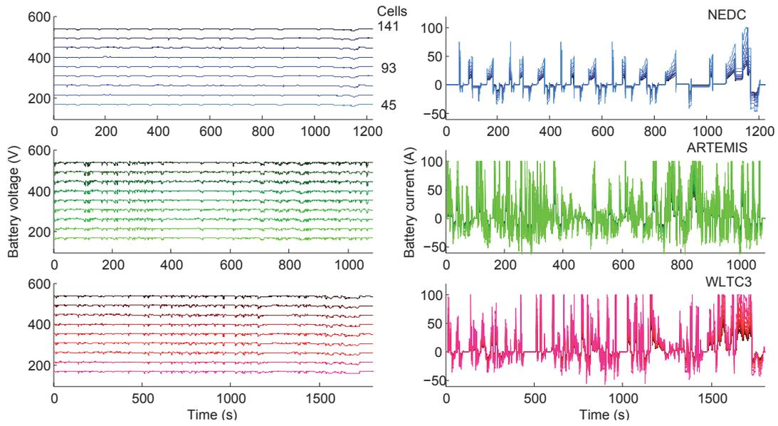
Figure 5.17: Battery voltage and current response for the three road cycles; NEDC, ARTEMIS, and WLTC3 if the number of battery cells are reduced.
