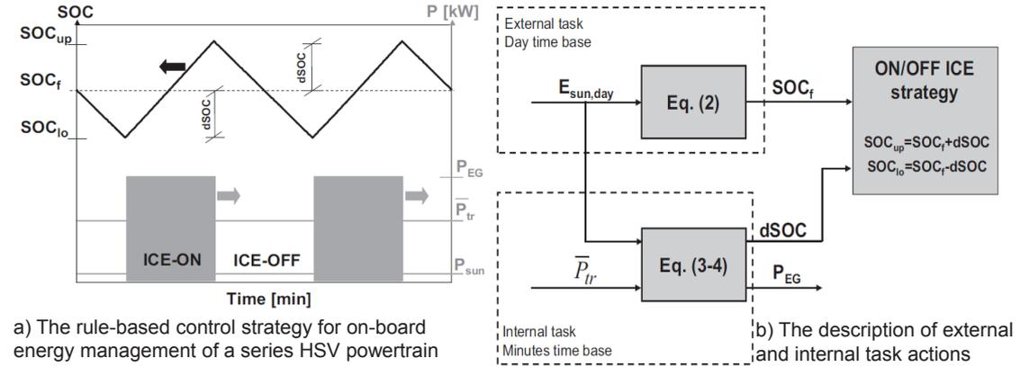
Figure 2.10: Schematic representation of; a) The rule-based control strategy for on-board energy management of a series HSV powertrain, and b) The description of external and internal task actions [72].
