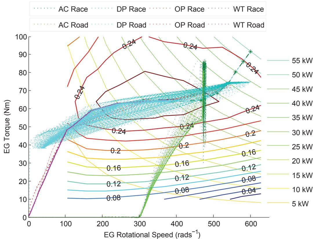
Figure 5.9: Distribution of speed and torque of the generator on the EG map of all cycles under all four control strategies.
