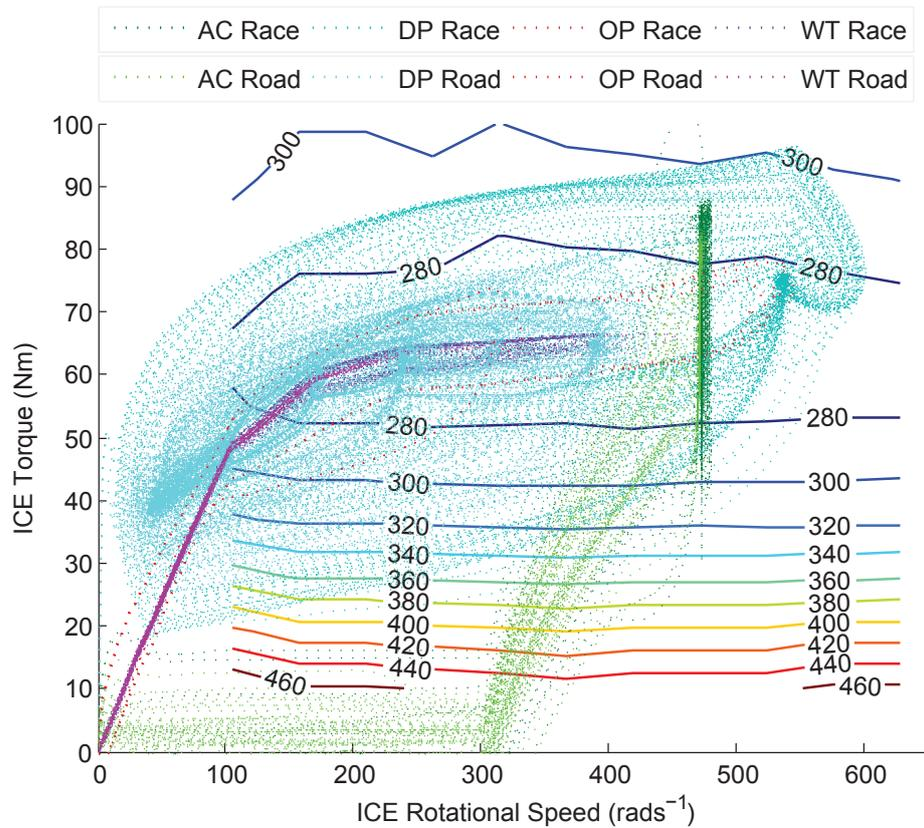
Figure 5.8: Working points of the engine on the BSFC map of all cycles under all four control strategies.
