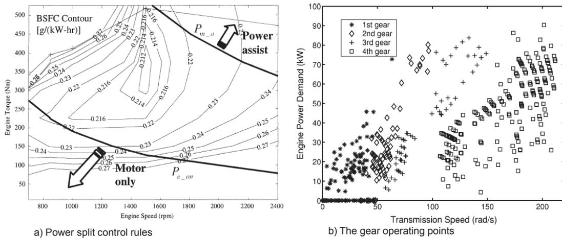
Figure 2.27: The DP optimisation; a) Power split control rules, and b) The gear operating points [42].
