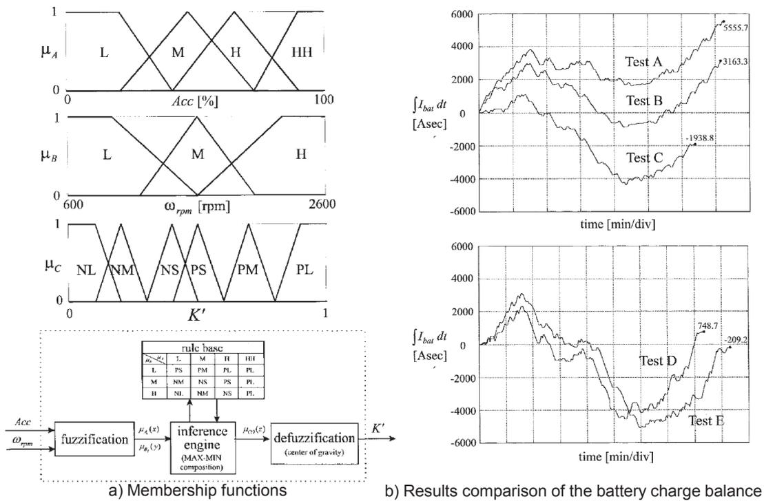
Figure 2.12: The fuzzy rules control strategy; a) Membership functions, and b) Results comparison of the battery charge balance [22].
