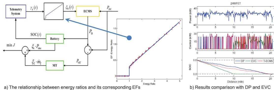
Figure 2.37: Schematic illustration of T-ECMS; a) The relationship between energy ratios and its corresponding EFs, and b) Results comparison with DP and EVC [9].
