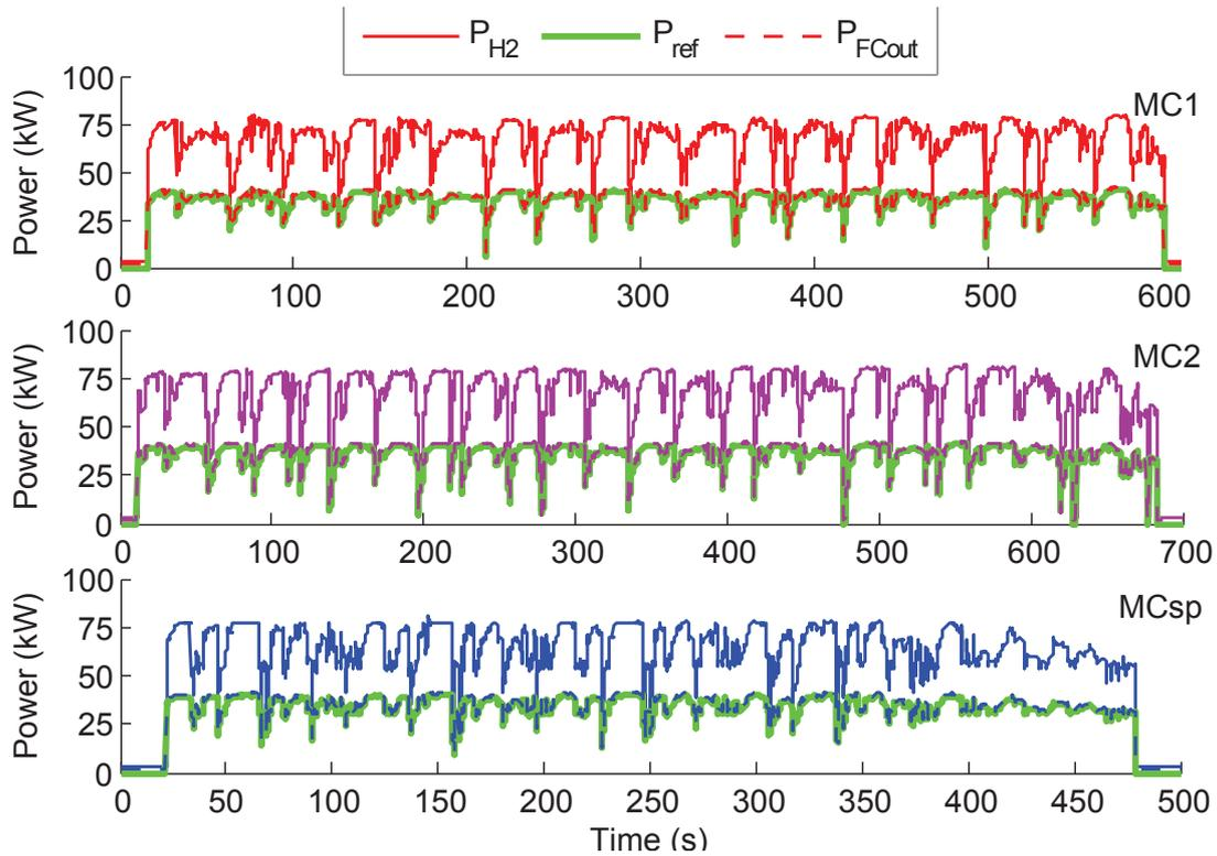
Figure 3.26: Comparison between the demanded reference power and the fuel cell power for MC1, MC2, and MCsp driving cycles.
