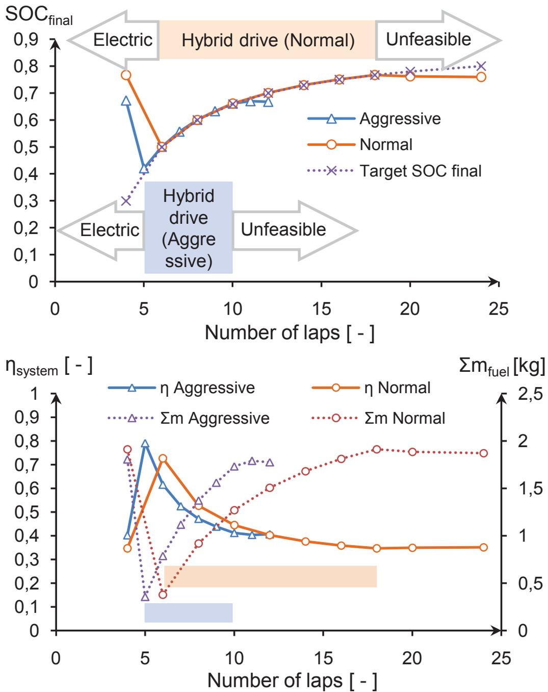
Figure 4.9: DP Optimisation limits for the two studied driving cycle.
