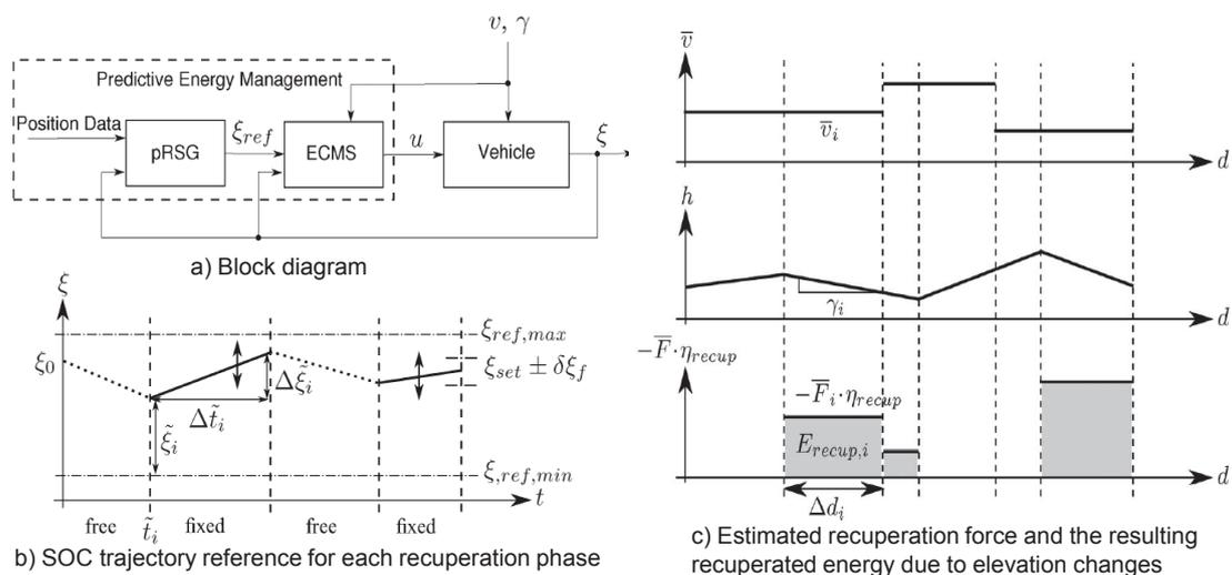
Figure 2.35: The concept of the pRSG-ECMS control strategy; a) Block diagram, b) SOC trajectory reference for each recuperation phase, and c) Estimated recuperation force and the resulting recuperated energy due to elevation changes [68].
