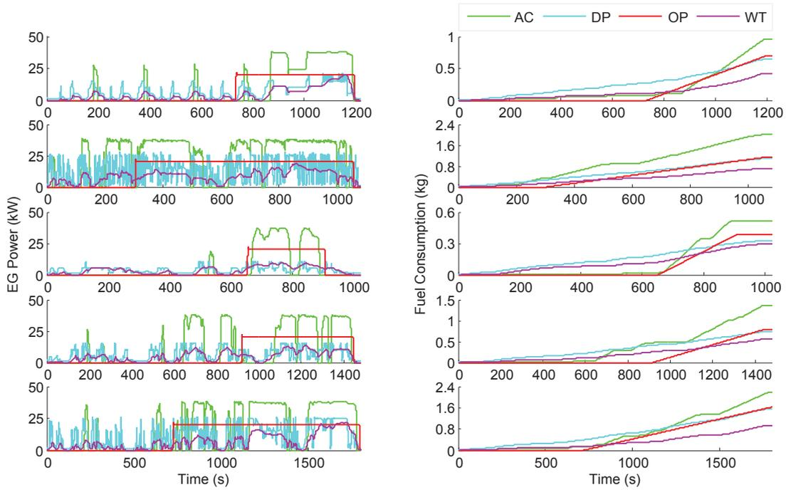
Figure 5.7: Results comparison of the EG power and fuel consumption of the road cycles (NEDC, ARTEMIS, WLTC1, WLTC2, WLTC3) for all four control strategies.
