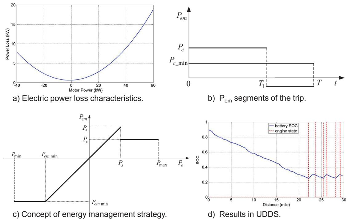
Figure 2.11: Illustration of the control strategy method; a) Electric power loss characteristics, b)  $P_{em}$  segments of the trip, c) Concept of energy management strategy, and d) Results in UDSS [29].
