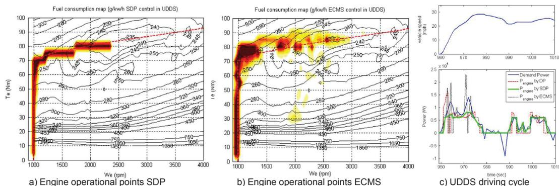
Figure 2.30: Results of the control strategies; a) Engine operational points SDP, b) Engine operational points ECMS, and c) UDDS driving cycle [74].
