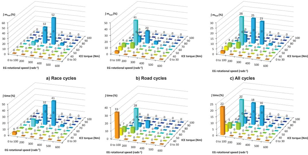
Figure 5.14: Percentage of ICE points distribution for the optimal torque control in terms of fuel consumption and time spent.
