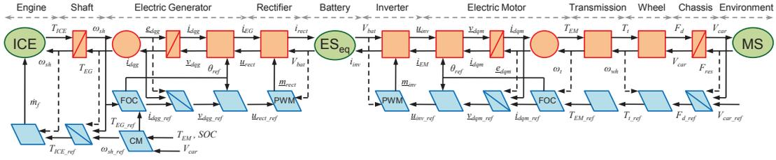
Figure 3.12: Energetic Macroscopic Representation of the car system and its control scheme with the equivalent electrical source.
