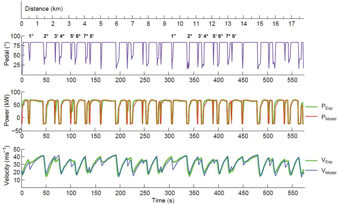
Figure 4.14: Comparison of the model with results from experiment for the Grand Prix circuit.
