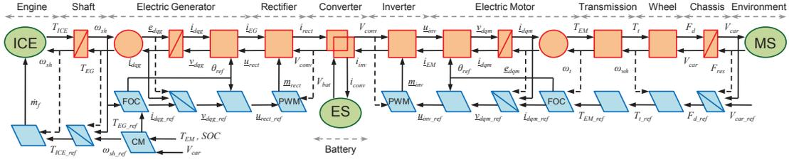
Figure 3.11: Energetic Macroscopic Representation of the car system and its control scheme.
