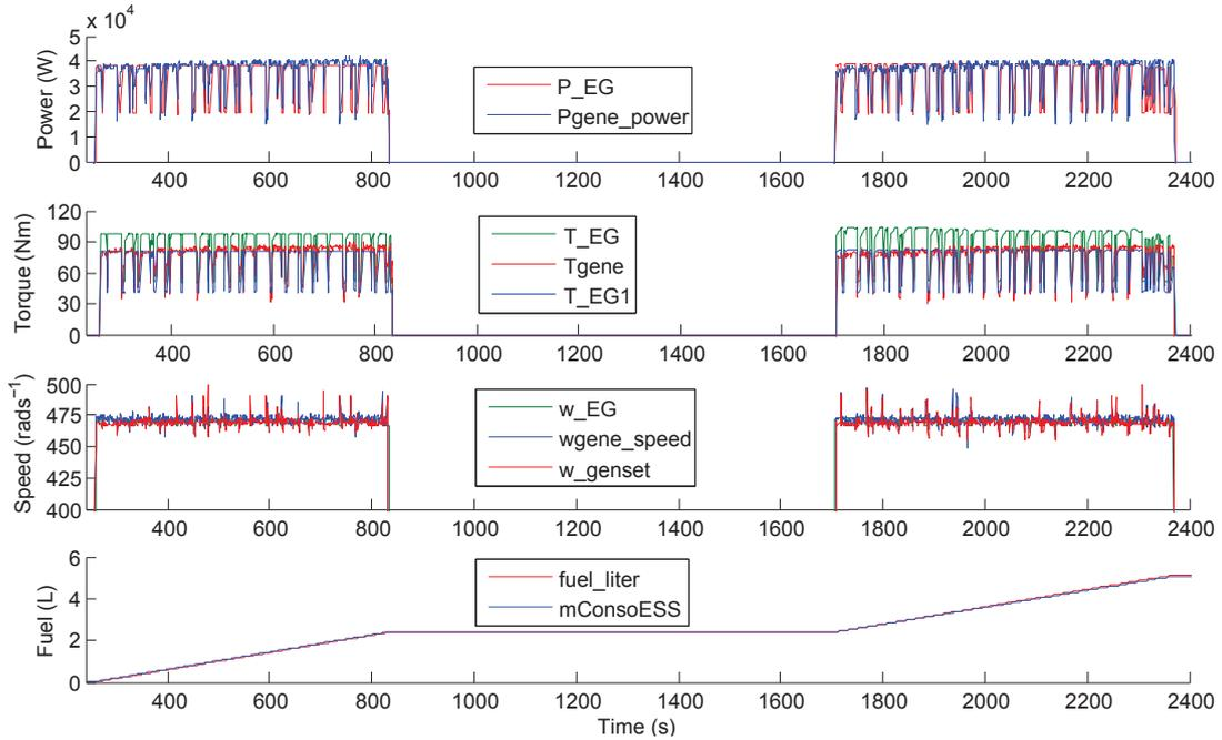
Figure 3.10: Verification of the engine and generator model of the Noao car using quasi-static modeling method.
