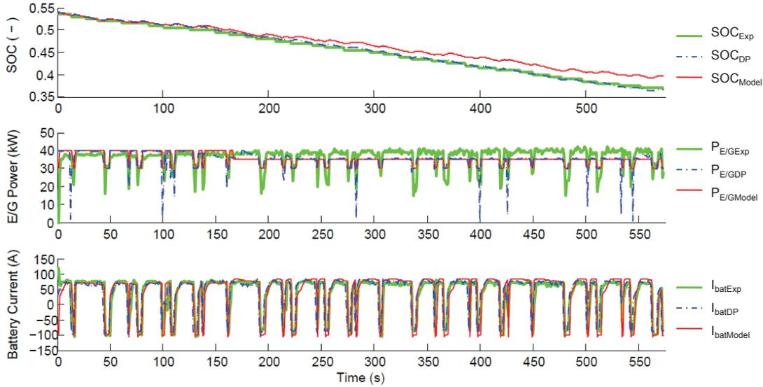
Figure 4.10: Comparison of SOC evolution and the systems power distribution for the experiment, optimization using DP, and the adjusted controller.
