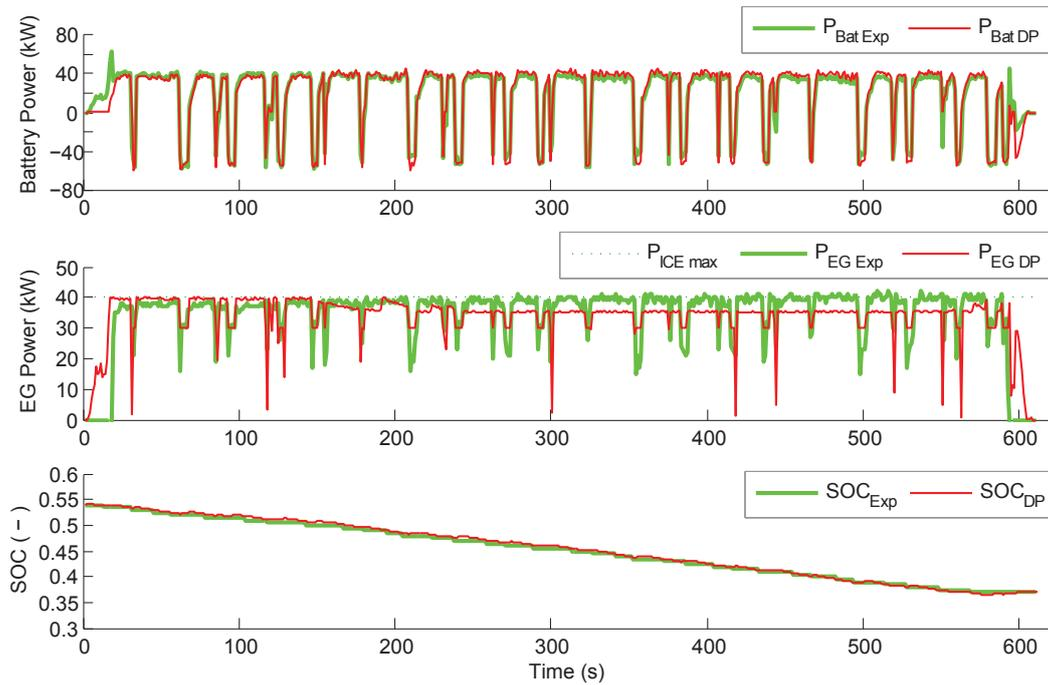
Figure 4.4: DP optimisation of the MC1 driving cycle.
