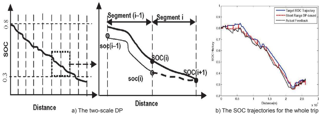
Figure 2.29: Comparison of; a) The two-scale DP, and b) The SOC trajectories for the whole trip [96].
