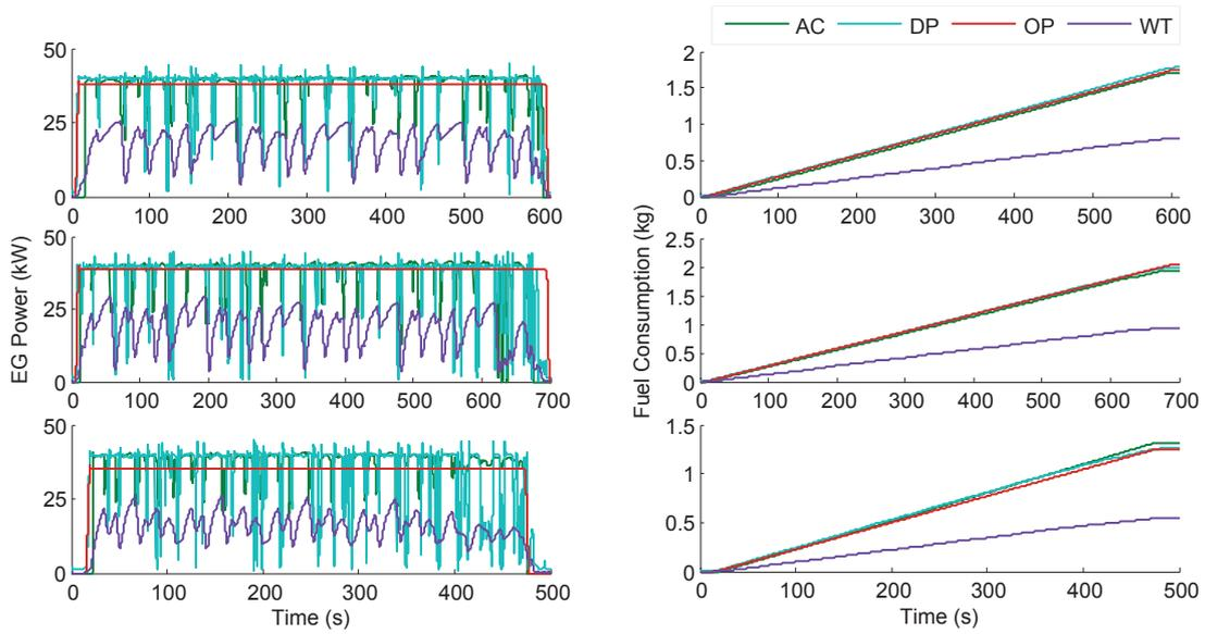
Figure 5.5: Results comparison of the EG power and fuel consumption of the race cycles (MCNoao1, MCNoao2, MCNoaosp) for all four control strategies.
