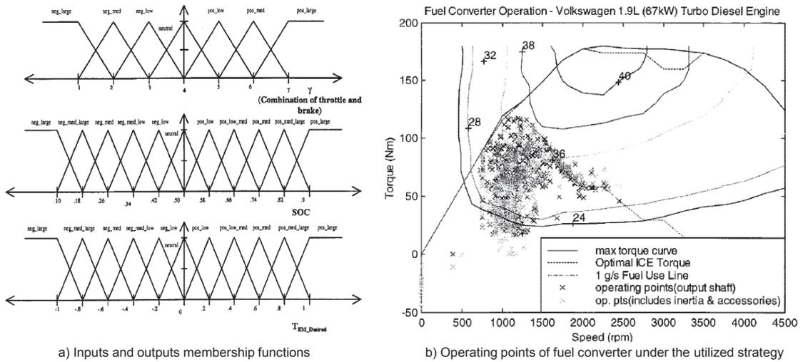
Figure 2.13: Fuzzy logic controller; a) Inputs and outputs membership functions, and b) Operating points of fuel converter under the utilized strategy [1].
