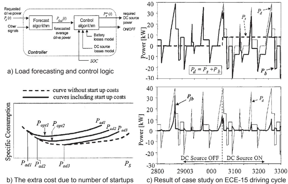
Figure 2.5: The control method; a) Load forecasting and control logic, b) The extra cost due to number of startups, and c) Result of case study on ECE-15 driving cycle [50].
