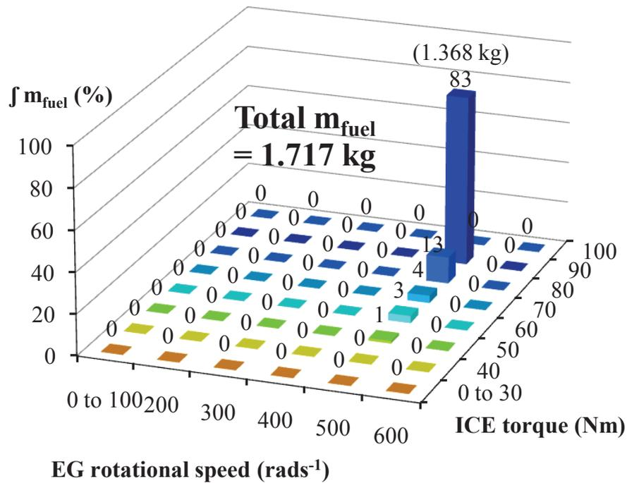
Figure 3.19: Percentage of the engine fuel consumption using the actual control parameters.
