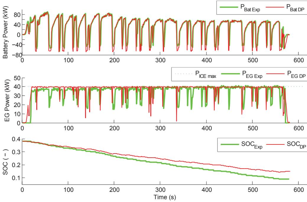
Figure 4.7: DP optimisation of the MC2, a more aggressive driving cycle of MC1 for a longer autonomy.
