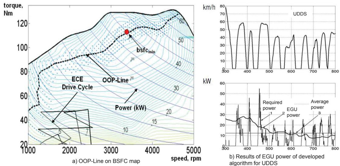
Figure 2.20: The concept of the control; a) OOP-Line on BSFC map, and b) Results of EGU power of developed algorithm for UDDS [92].
