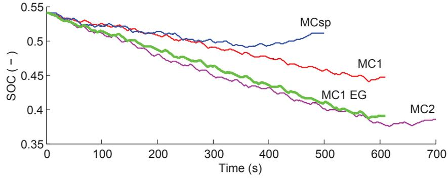
Figure 3.27: SOC evolution of the battery by using the fuel cell stack as range extender in the racing car system for MC1, MC2, and MCsp driving cycles.
