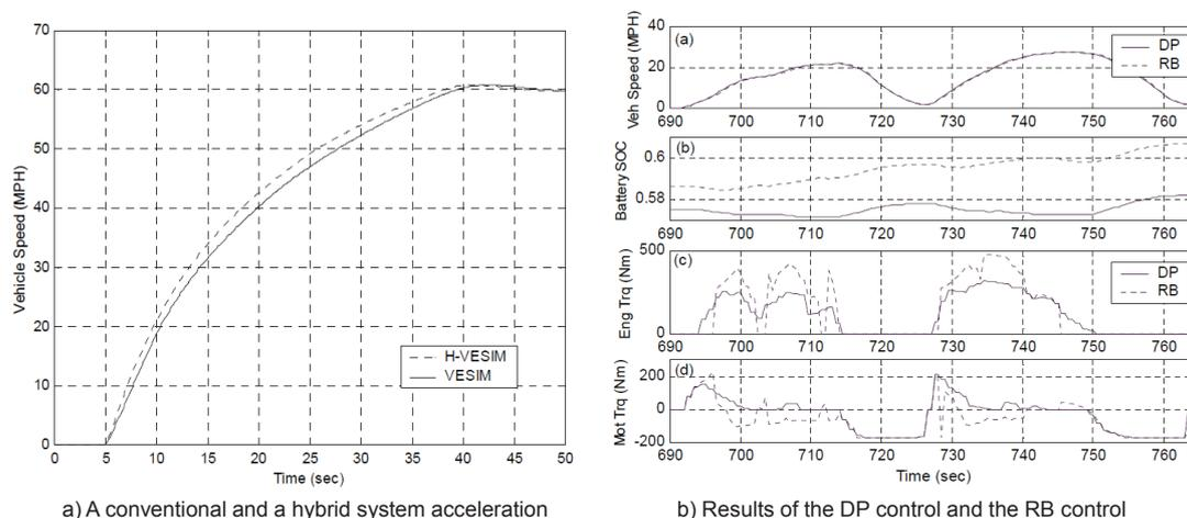
Figure 2.25: Comparison of; a) A conventional and a hybrid system acceleration, and b) Results of the DP control and the RB control [8].
