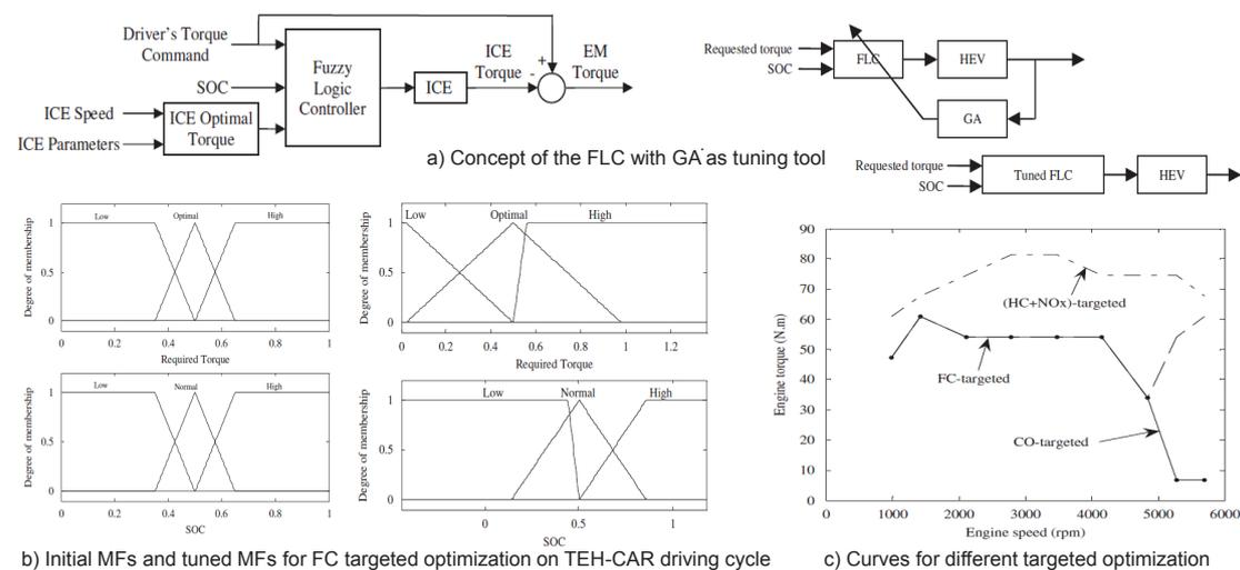
Figure 2.16: The fuzzy logic controller (FLC); a) Concept of the FLC with GA as tuning tool, b) Initial MFs and tuned MFs for FC targeted optimization on TEH-CAR driving cycle, and c) Curves for different targeted optimization [85].
