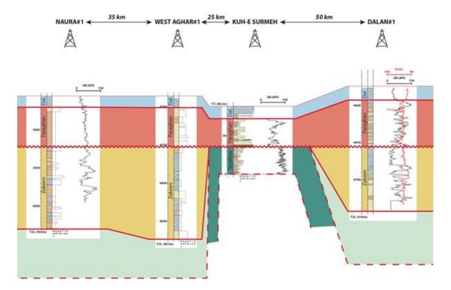
**Fig. V.7:** Stratigraphic correlation between Kuh-e- Surmeh, Naura#1, West Aghar#1, and Dalan#1. Evidenced of a large hiatus between Ordovician Seyahou and Permian Faraghan Fms in Kuh-e Surmeh where the Devonian Zakeen Fm. is lacking but well recorded in the other drilled sections.
