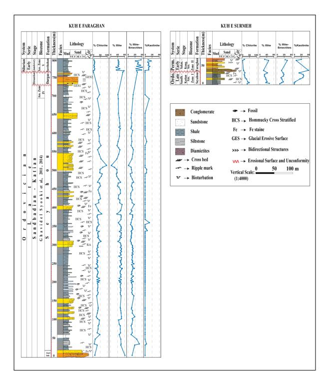
**Fig. IV.3:** Lithology vs. Chlorite, Illite, Illite/ Smectites and Kaolinite for the Zard Kuh, Seyahou and Dargaz Formations in Kuh e Faraghan and Seyahou Fomation in Kuh e Surmeh. *For the facies color codes see table IV.1&2*
