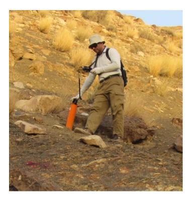
Fig. II.2: Measurement of gamma-ray with GS-512.
