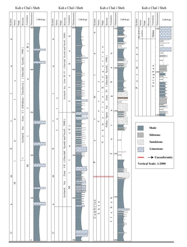
Fig. III.5: Litho-stratigraphic log of Chal i Sheh (modified after JOGMEC & NIOC, 2005).
