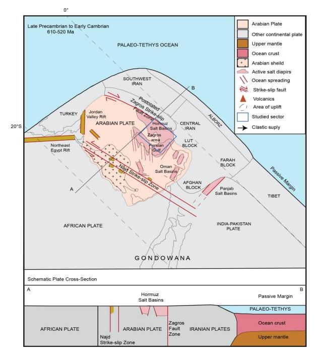
**Fig. I.5:** Schematic plate reconstruction and cross-section for Late Pre-Cambrian to Early Cambrian (Sharland et al., 2001). Hormuz Salt basins in Zagros activated since Palaeozoic age (Jahani et al., 2009).
