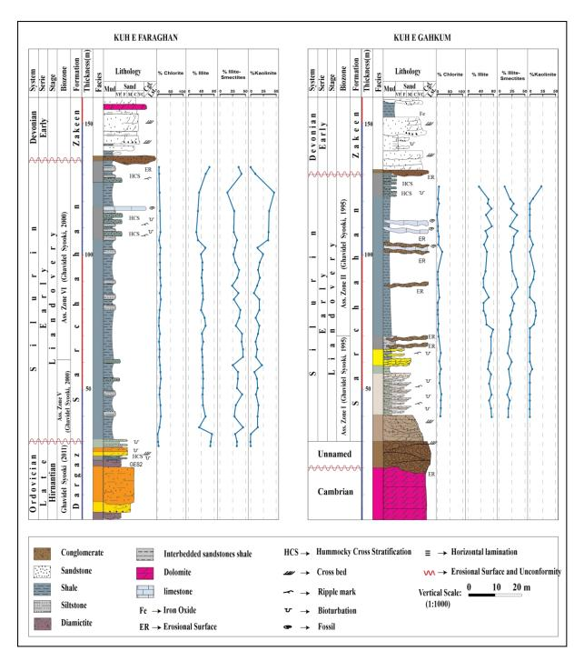
**Fig. IV.14:** Lithology vs. Chlorite, Illite, Illite/ Smectites and Kaolinite for the Sarchahan Formation in Kuh e Faraghan and Kuh e Gahkum outcrops. *For the facies color codes see table IV.3*.
