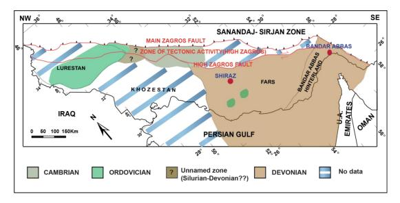
**Fig. V.6:** Hercynian subcrop map in the Zagros area. Occurrences of Devonian sequences are preserved under the Hercynian unconformity in Fas and Bandar Abbas areas. In other areas of the Zagros (e.g. Wast High Zagros), the Silurian, Devonian and Carboniferous are largely missing and older Palaeozoic rocks subcrop under the unconformity.
