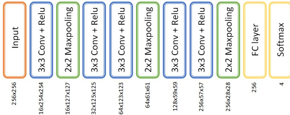
Fig. 57: Architecture of the CNN model. The input layer accepts B-scans with 256x256 pixels from CUHK dataset. The parameters (feature maps and size) are reported beneath every layer.
