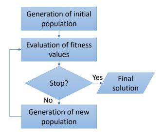
Figure 5.1: Flowchart of an evolutionary algorithm
