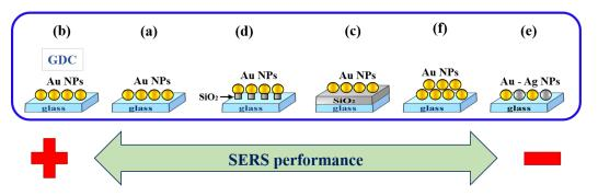
Fig. 2.13: Schematic representation of SERS substrates. Au nanoparticle substrate (a) without and (b) with glow charge cleaning (GDC). Au nanoparticles on (c) silica layer and (d) silica pillars. (e) Au-Ag bimetallic and (d) twice deposited Au nanoparticle substrate. Scale bar is 100 nm for all SEM images.
