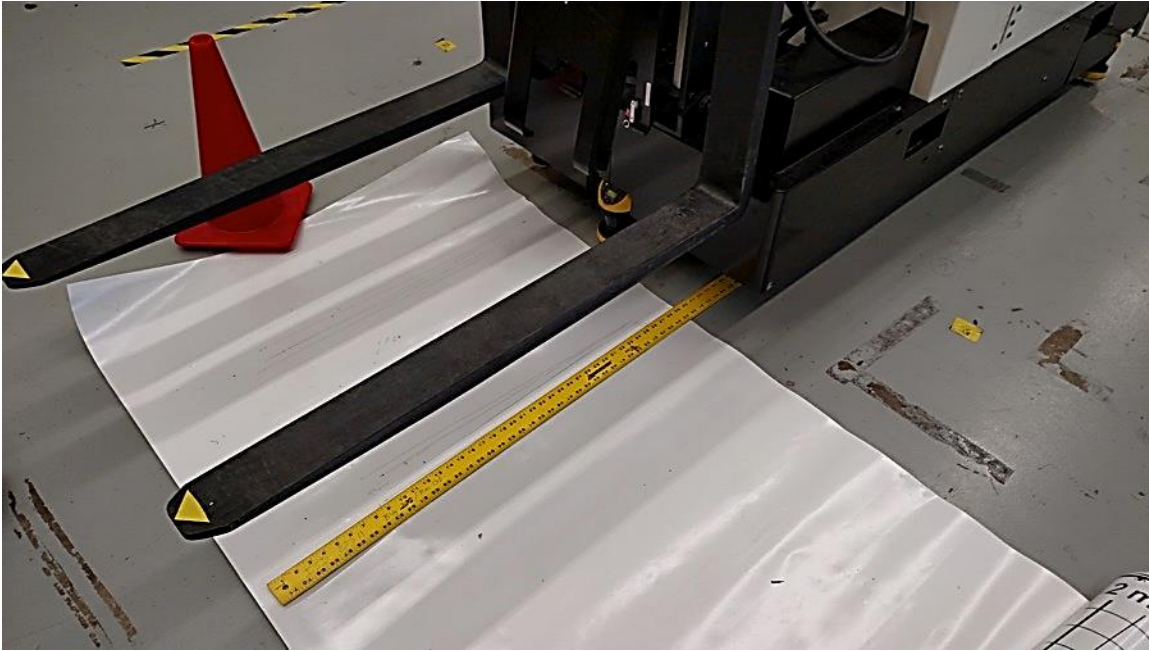
Figure 37. Marking out toe-in angle on a sheet of paper.
