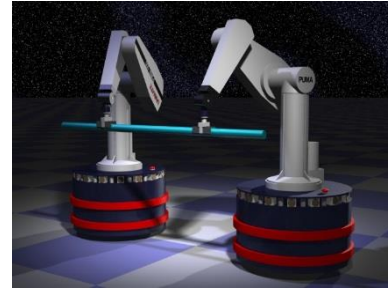
Figure 4. Graphical depiction of the Stanford Assistant Mobile Manipulators (SAMM) carrying a pipe.
