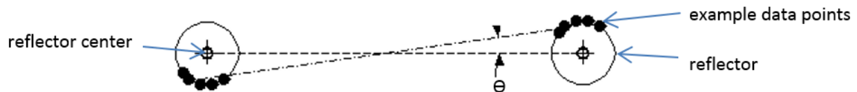
Figure 29. Graphic of possible orientation uncertainty when the reflector center is not detected.
