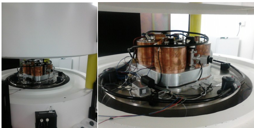
Figure 5: Cyclotron 7.5 MeV ABT Biomarker Generator cyclotron (ABT Molecular Imaging, Inc. ©, USA) de l'Université de Hull
