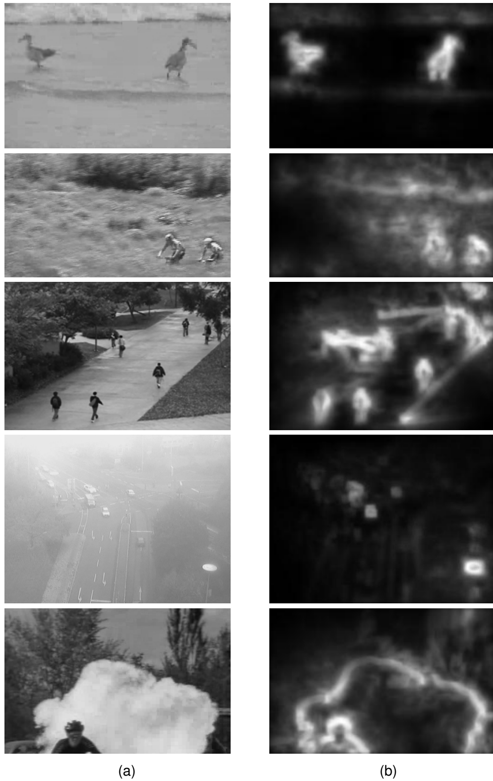
FIGURE 3.2 – Examples of static saliency detection. (a) Original frame (b) Static saliency map.
