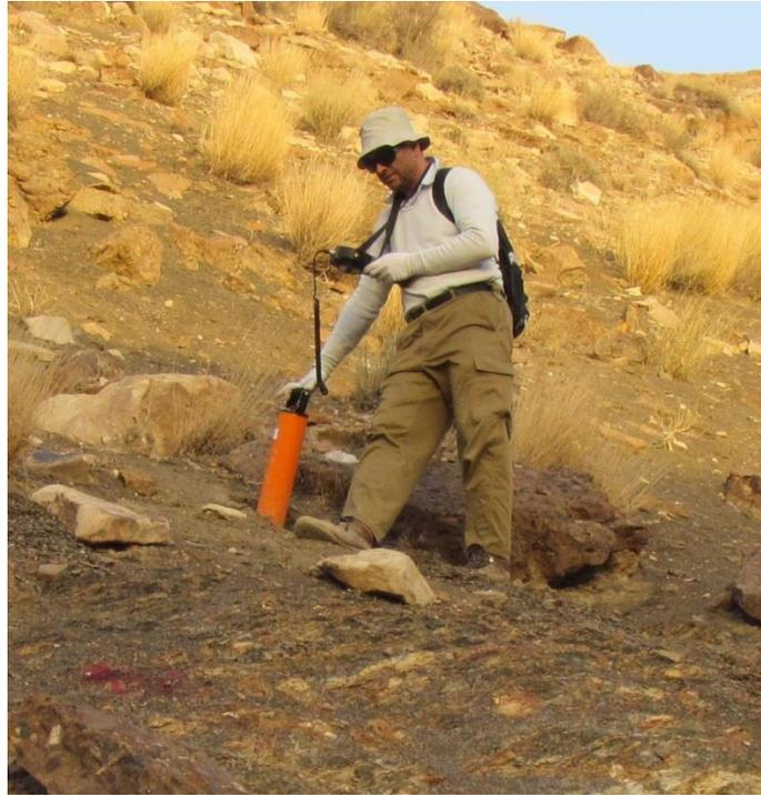
**Fig. II.2:** Measurement of gamma-ray with GS-512.
