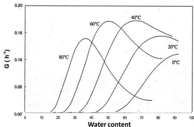
Figure 39 : Influence of water content and storage temperature exerted on wheat starch isothermal re-crystallization as illustrated by the Lauritzen–Hoffman simulation (the dependence of the rate of retrogradation at a constant storage temperature on the water content was attempted using this latter theory) (Farhat et al., 2000).
