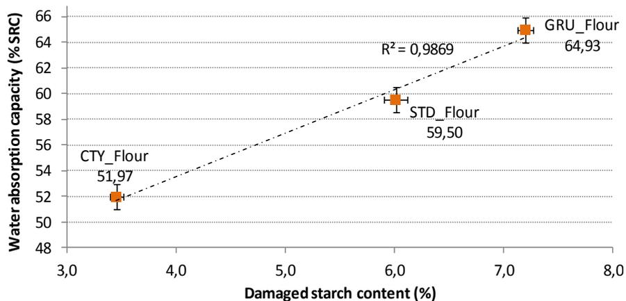
Figure 79 : SRC water absorption capacity as a function of the flour damaged starch content (%). The linear curve represents the evaluated correlation between the mean values obtained for three different types of flour.
