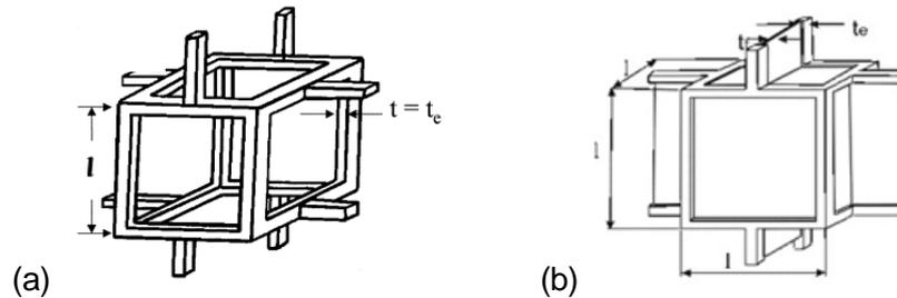
Figure 10 : Cellular solids cell representation (unit cells drawn as cubes, so that  $l=h$ ): a statement of whether it is open (a) or closed (b). Most of them behave like open-cell foams. Adapted from (Ashby & Medalist, 1983).
