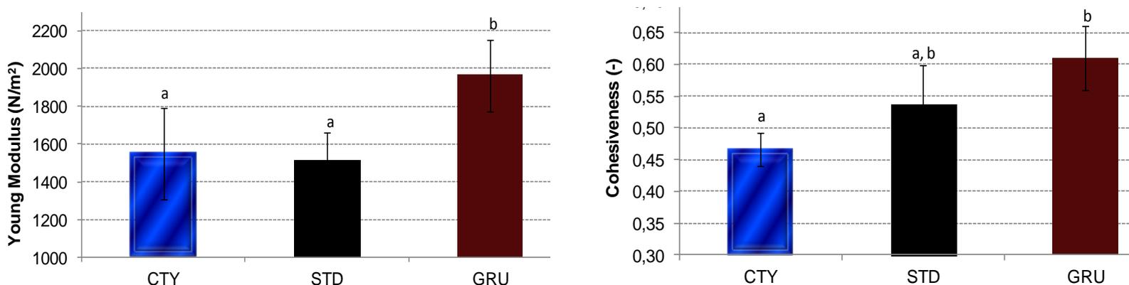
Figure 83 : Impact of flour nature on several cake sample textural properties (Young modulus left; cohesiveness, right). Measurements were driven using a TAXT<sub>2</sub> texturometer under compression. While sample deforms (% compression distance), the response is recorded as the resulting force responses.
