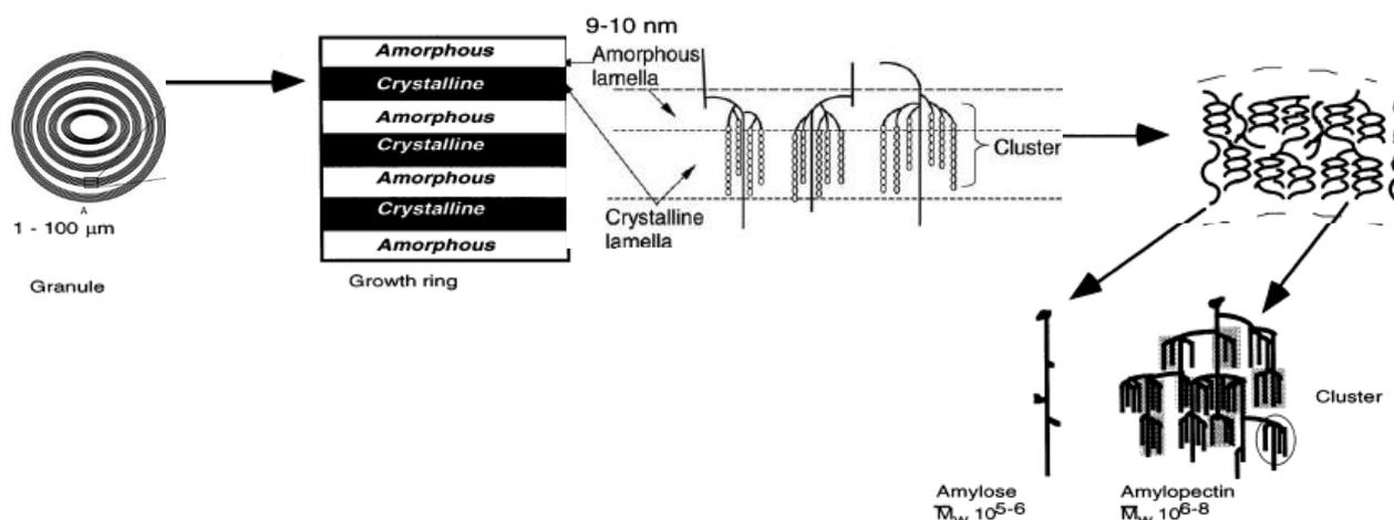
Figure 31 : Representation of the starch granule at different structure levels: adapted from (Buléon et al., 1998, Tester et al., 2004).
