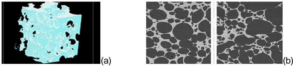
Figure 12 : Structure of aerated cereal solid (bread-like sample) observed by X-Ray Tomography: (a) 3D representation of an aerated baked cereal solid (Della Valle, 2006) and (b) 2D sections of a 3D image of bread crumb (Lassoued et al., 2007).
