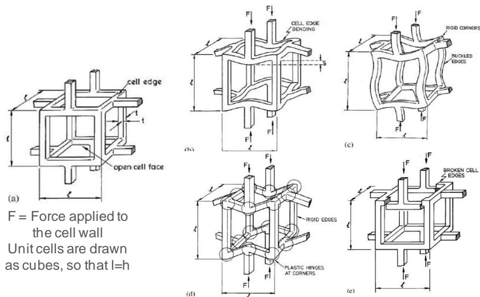
Figure 17 : Illustration of the three mechanical behavior models: idealized undeformed cell in an open-cell foam (a), elastic foam under linear elastic bending (b); elastomeric (c) elastic-plastic (d), and brittle foam (e) under uniaxial compression ( $F$  value) using an Instron testing machine: (Gibson, 2005).
