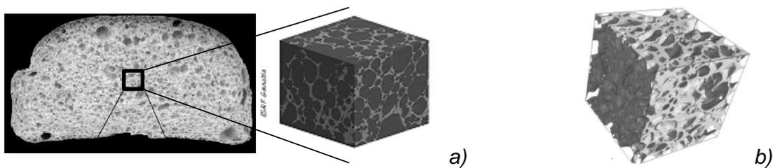
Figure 14: Aerated cereal product structure model; piece of bread crumb reconstruction from its X-Ray Tomography 3D scan image : a) Sphere packing approach (Lassoued, 2005, Lassoued et al., 2007); b) matrix continuity with closed cells connections (Maire et al., 2003).
