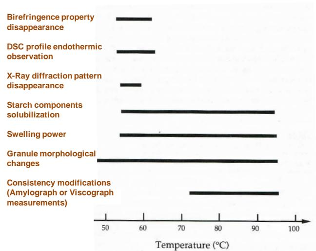
Figure 32 : Temperature range and phenomenon taking place while starch granules are heated with an excess of water during gelatinization: from (Eliasson & Larsson, 1993).
