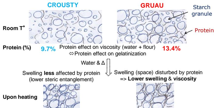
Figure 95 : CTY and GRU flour at ambient temperature then upon heating: wheat flour proteins impact on starch swelling.
