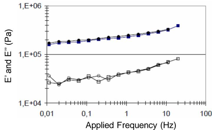
Figure 19: E' (black markers) and E'' (white circle and square) modulus values evolution as a function of the applied frequency. Measurement was performed at 25°C with a strain rate of  $9.10^{-3}\%$  on two equivalent bread crumb samples.
