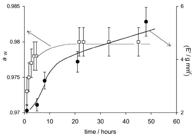
Figure 37 : Evolution of the Water Activity ( $a_w$ , left axis) and the Elastic modulus ( $E'$ , right axis) as a function of time in the early staling phenomenon phases of a bread crumb stored at room temperature (Pavinee & Vodovotz, 2001).
