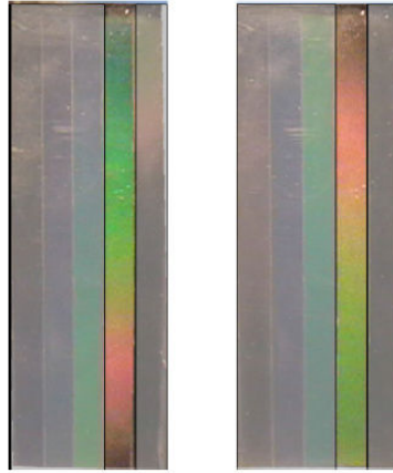
Figure 21. Left: temperature visualization 18 min at 6C test without cooling. Right: the same image 34 min into the test with cooling [77].
