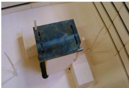
Figure III. 13 Gas module aligned with ceramic tubes
