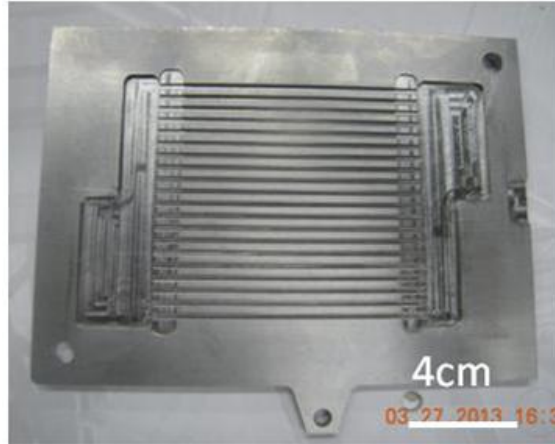
Figure III. 9 Interconnector with serpentine flow pattern
