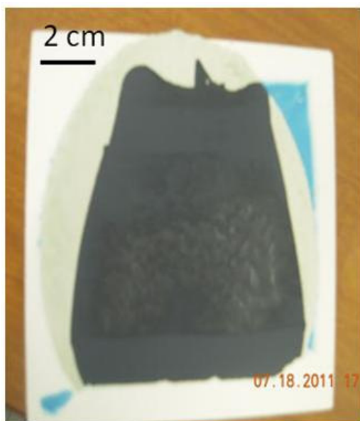
Figure II. 17 Full cell by only tape casting Figure II. 18 Sintering protocol for cathode layer
