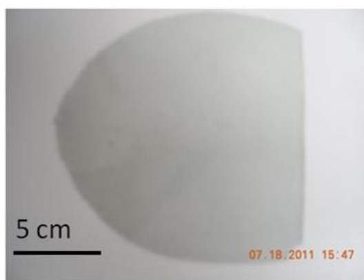
Figure II. 16 Sintered half cell
