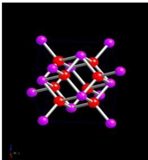
Figure II. 1 GDC crystal structure drawn by Topaz software
