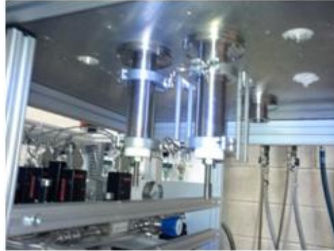
Figure III. 14 Bottom plates with D40 flanges
