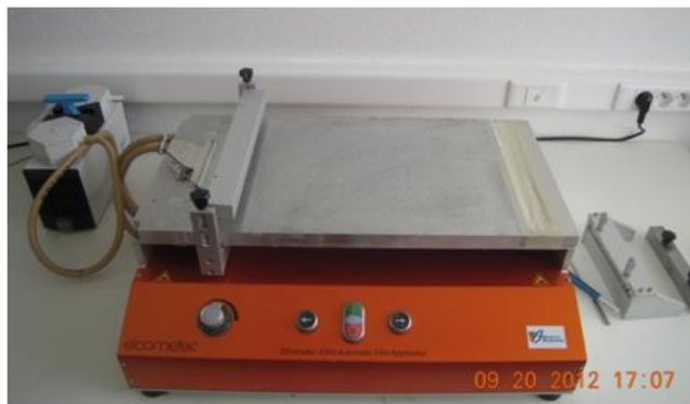
Figure II. 11 Automated tape casting machine
