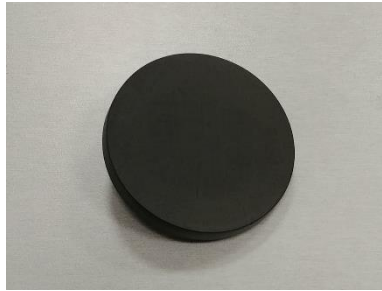
Figure 3.5 Black support used behind sample leaves during reflectance data acquisition.
