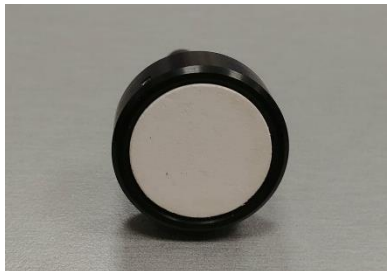
Figure 3.4 White reference used for calibration.
