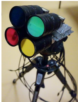
Figure F.1 Designed MS test sensor consisting of four identical IDS cameras equipped with 16 mm lens and four different filters {530, 63, 740, 810 nm} chosen for FD disease detection.
