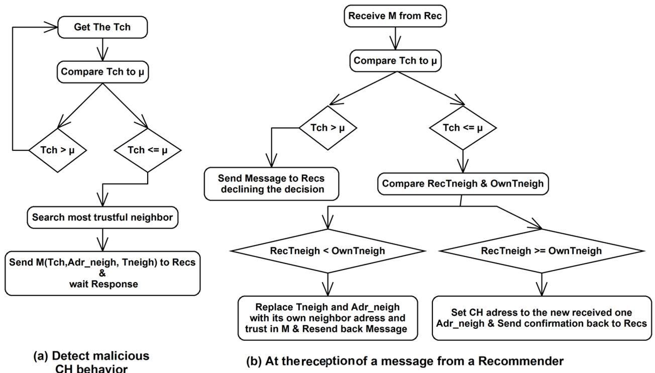
Figure 4.11 – CH Malicious behavior detection and replacement
