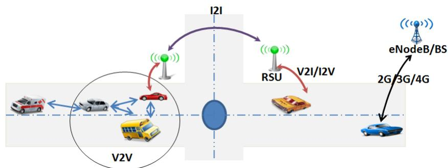
Figure 4.1 – Data collection in a vehicular network
