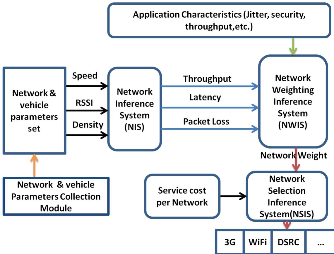
Figure 5.9 – The fuzzy-based network selection architecture
