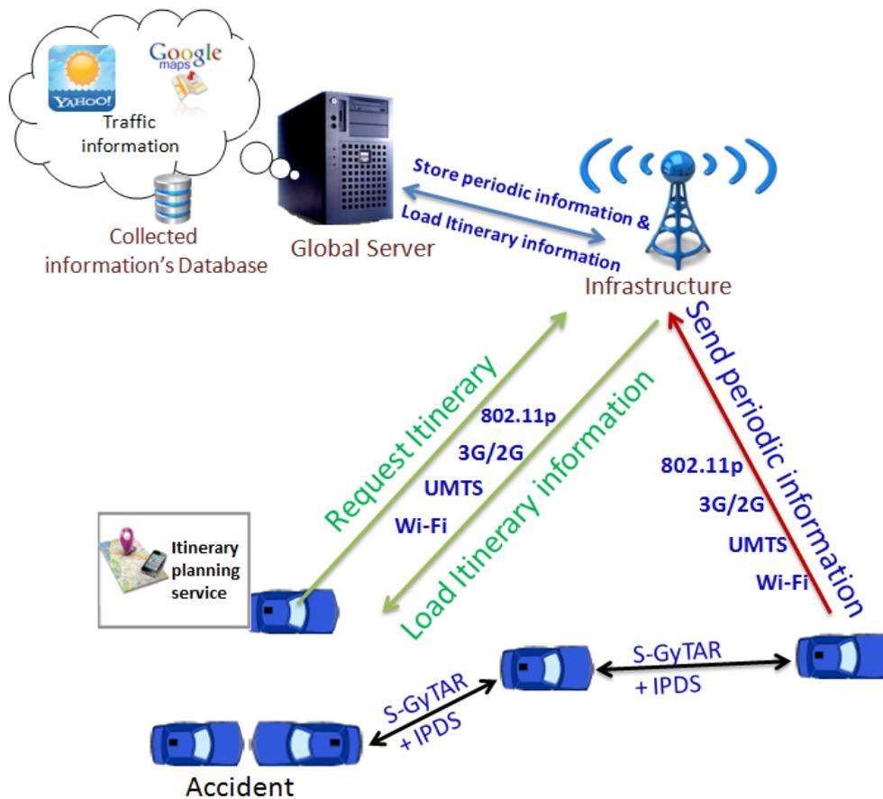
Figure 5.2 – Simplified architecture for Itinerary Planning service
