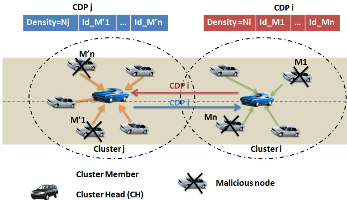
Figure 4.3 – Cluster monitoring & information exchange in S-GyTAR
