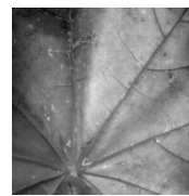
(d) Abundance map of first component, indicating the presence of chlorophyll in leaf.
