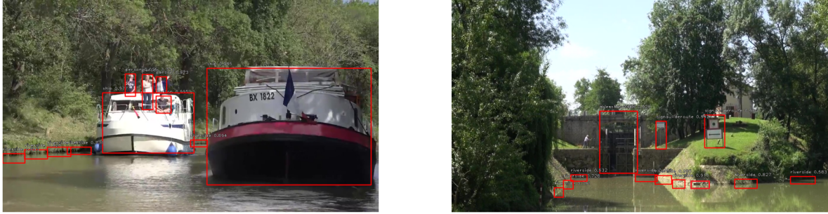
Figure 6.3: A sample of predicted images where the rectangles and text overlaid on the figures are the outputs generated by obstacle detection module.
