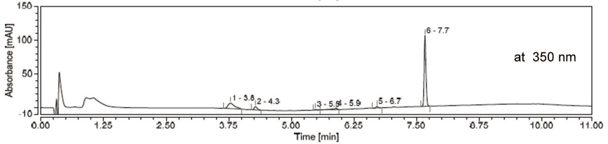
PLE-NTR probe **8** with NTR (0.6 U) and PLE (0.55 U) after 120 min
