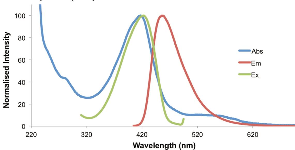
**Fig S3. Normalised absorption, excitation (Em. 530 nm) and emission (Ex. 370 nm) spectra of 3-cyano-7-hydroxycoumarin in PB at 25 °C.**
