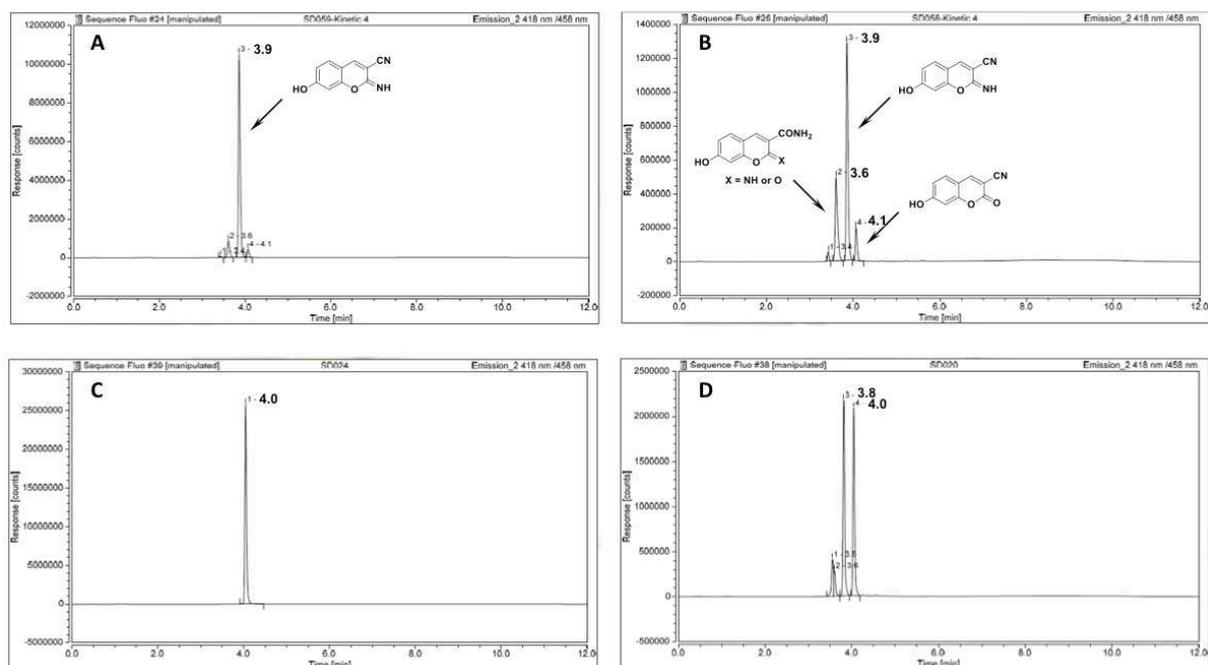
Enzymatic reaction mixtures (A-B) and authentic samples of 3-cyano-7-hydroxycoumarin (C) and 3-cyano-7-hydroxy-2-iminocoumarin (D). *Please note:* partial hydrolysis of cyano and imine moieties was occurred during HPLC analysis and incubation in PB. NADH ( $t_R = 3.4$  min) can be properly detected at a different wavelength channel (Ex./Em. 350/460 nm).
