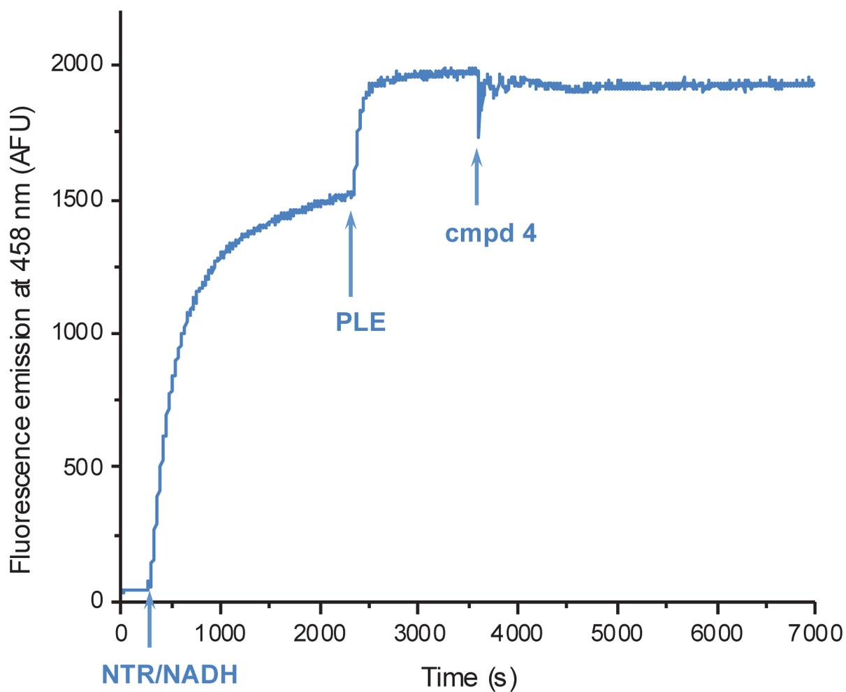
Probe **8** (concentration: 1.0  $\mu\text{M}$  in PB) was incubated with NTR (0.1 U) / NADH (45  $\mu\text{M}$ ) at 37  $^{\circ}\text{C}$  for 37.5 min, then PLE (1 U) was added and further incubation for 25 min. Finally, compound **4** (final concentration: 1.0  $\mu\text{M}$ ) was added. Ex./Em. 418/458 nm.
