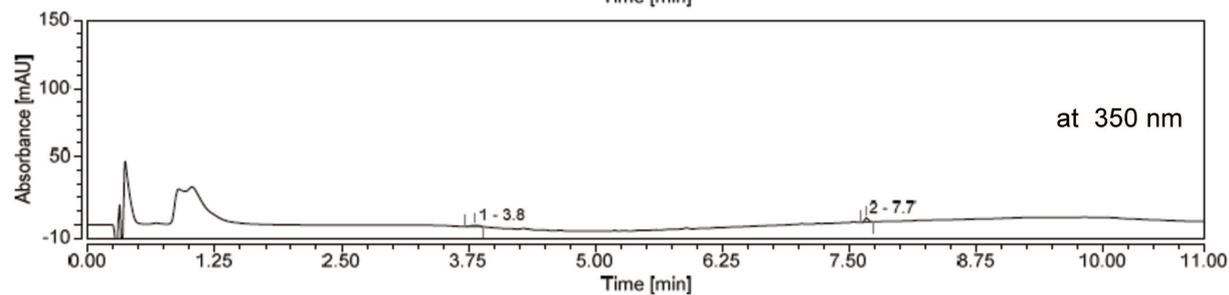
PLE-NTR probe **8** with NTR (0.6 U) after 120 min (addition of 0.55 U PLE at 80 min)
