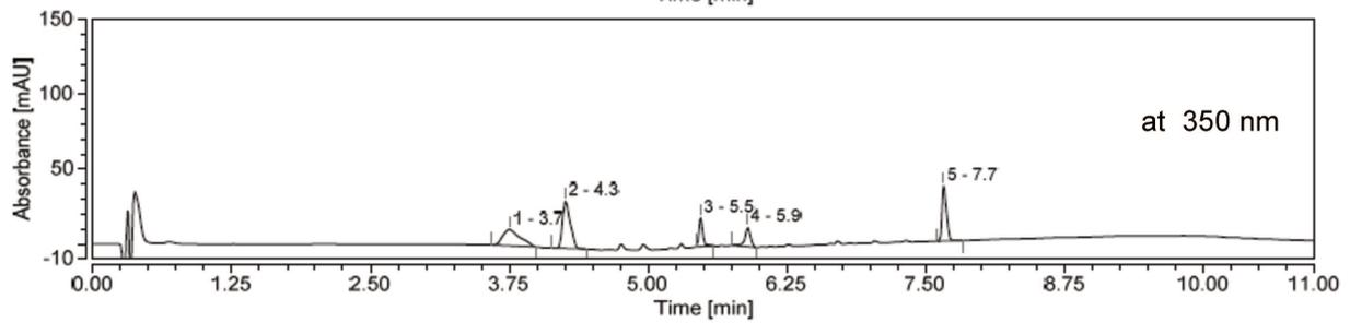
**Fig S12. RP-HPLC elution profiles (system C) of fluorogenic probe 9 after incubation in PB alone or with enzymes (PGA and NTR/NADH)**
