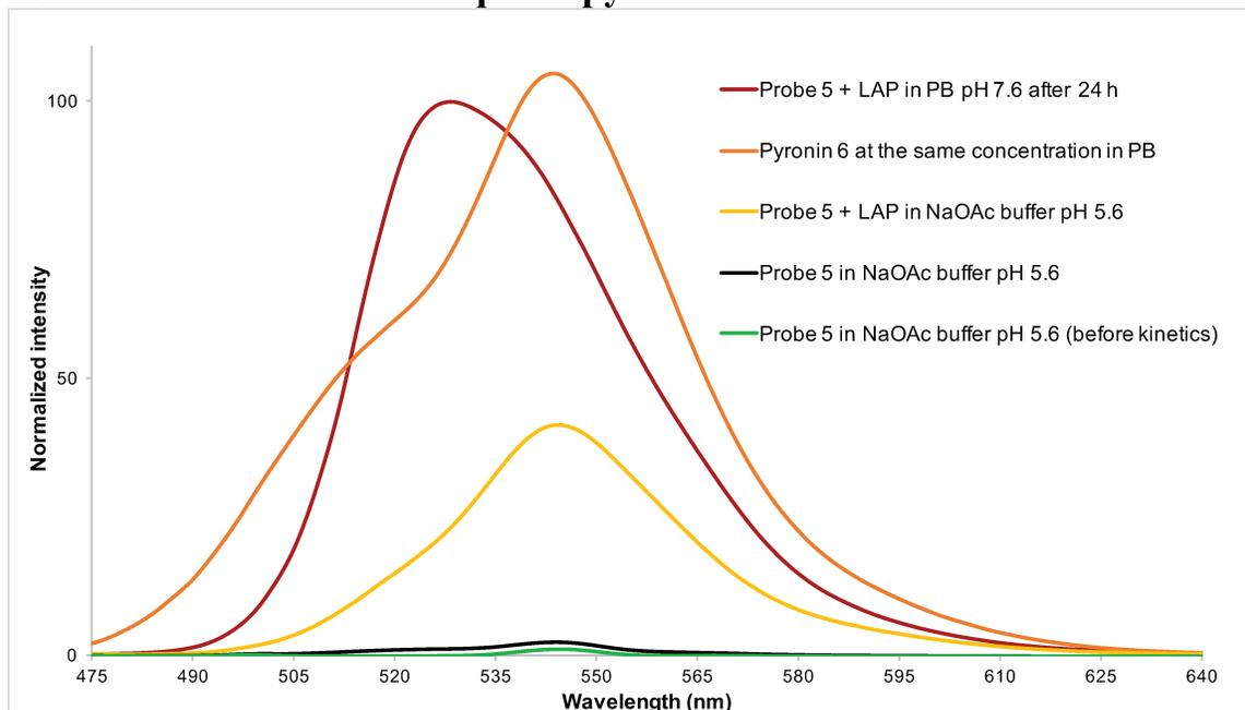
**Fig. S9** Overlaid fluorescence emission spectra (Ex. 460 nm, bandwidth 5 nm) of enzymatic reaction mixtures (probe 4) after 24 h of incubation at 37 °C
