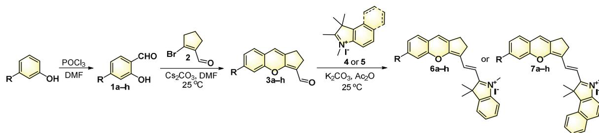
**Scheme S1.** General synthetic route towards *nor*-DHX-based fluorophores.
