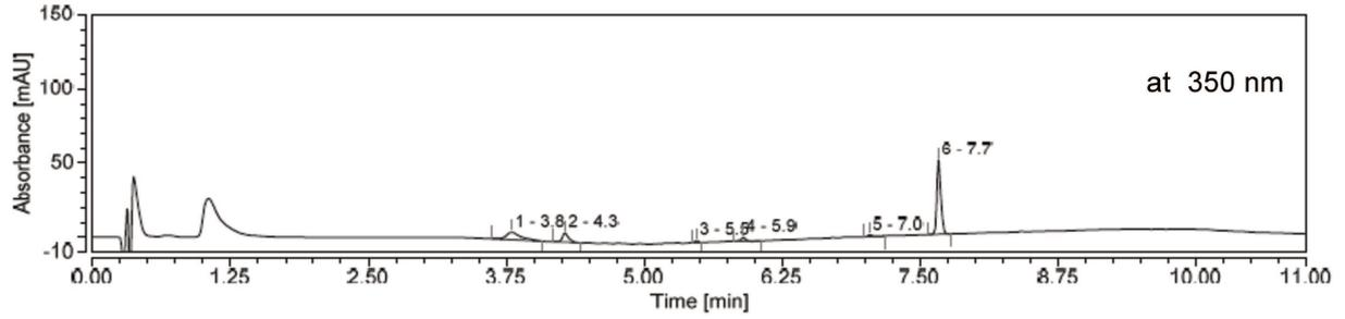
PLE-NTR probe **8** with NTR (0.6 U) after 180 min (addition of 0.55 U PLE at 80 min)
