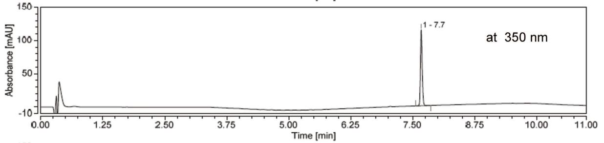
PLE-NTR probe **8** with PLE (0.55 U) after 120 min (addition of 0.6 U NTR at 80 min)
